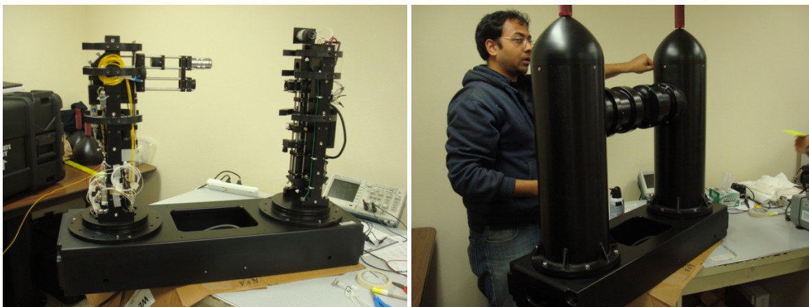
Figure 1. Internal electro-optical structure of the in-situ HOLOCAM (left panel). Pressure housings being assembled onto the first HOLOCAM (right panel).
