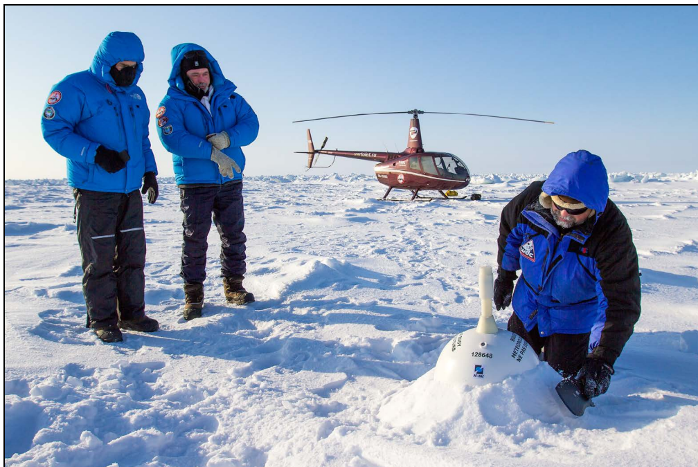
Figure 3. Deployment of an Marlin Yug SVP-B buoy in the Russian sector of the Arctic by Alexander Salman in April 2013. This buoy measures air pressure, surface temperature, and GPS positions.
