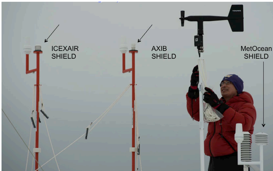
Figure 7. Air temperature sensor shields used by different manufacturers of buoys used by the IABP. How well do the different shields reduce solar heating of the sensor and reduce the bias in the air temperature measurement.
