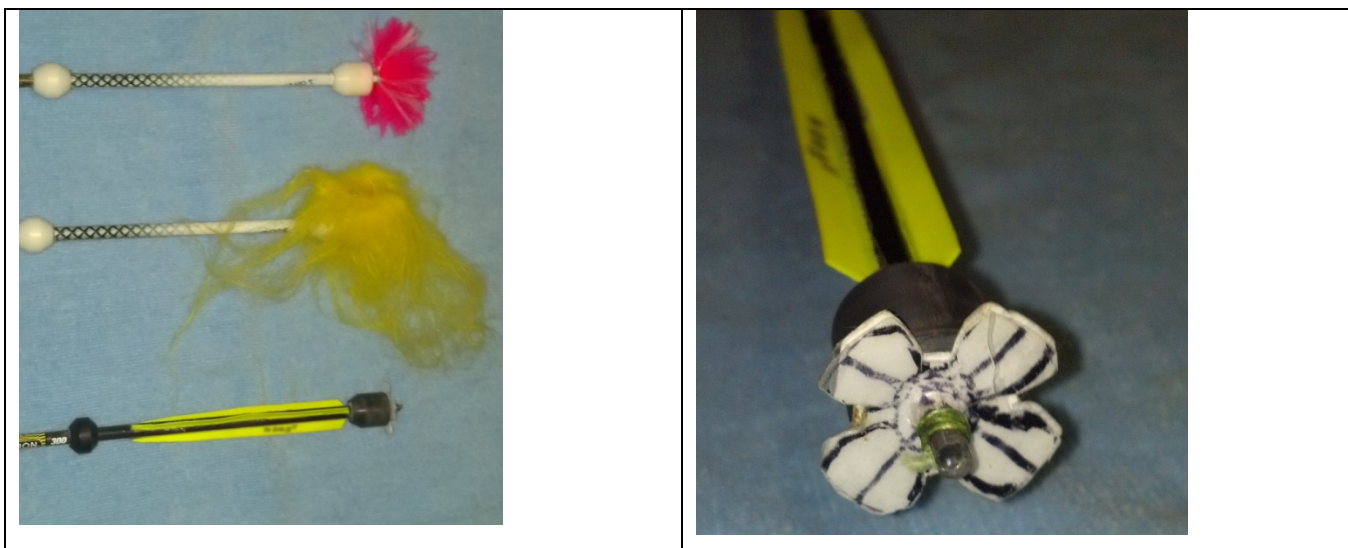
Fig. 8. Left: arrow end designs used in ballistics testing; from top to bottom; arrow m005, m006 and m007. Right: close up view of the end of arrow m007 showing the yellow vanes, similar to those found on crossbow bolts, and the addition of a plastic air brake that comes out proud of the end cap in flight.
