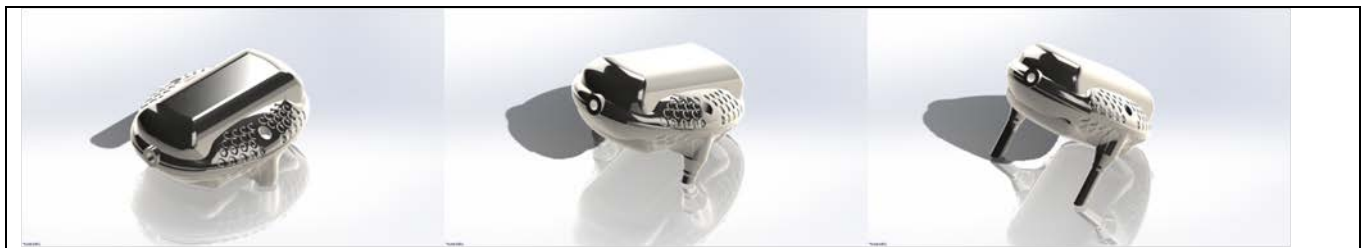
Fig. 4. Pitch angles of 0° (left), 20° (center), and 40° (right). Flow direction: lower left to upper right.
