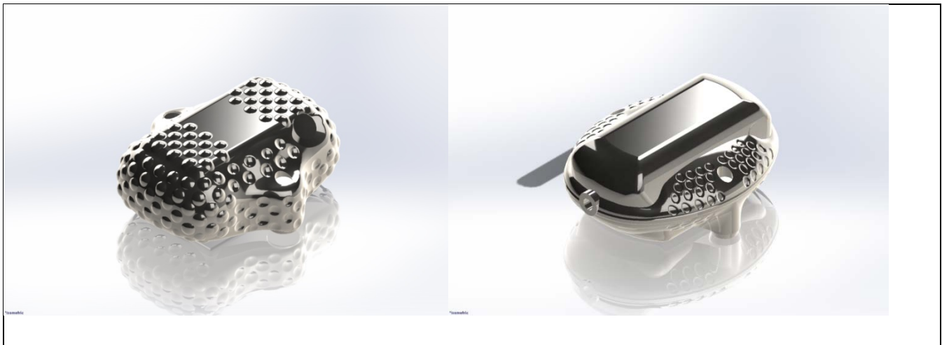
Fig. 1. CAD models of the most recent designs of the location-only LIMPET tag (AM-240C, Left) and the dive depth-transmitting LIMPET tag (AM-292, Right). The antennae and wet-dry sensors were removed to simplify the mesh
