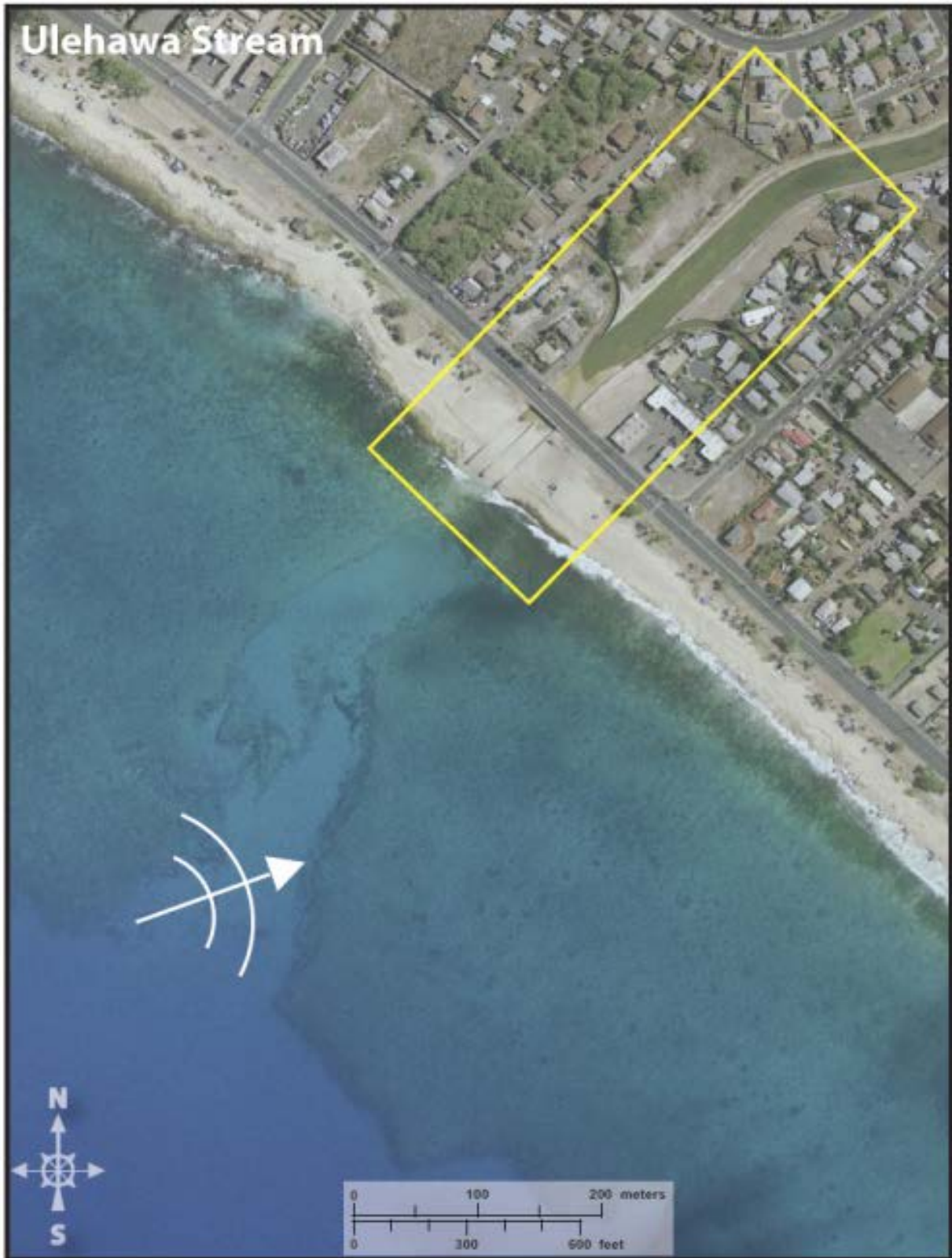
Figure 15. Aerial image of Ulehawa Stream showing sediment clogging the stream mouth.
