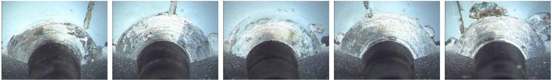
17 Weeks Wet Install with Primer Mag Rich
