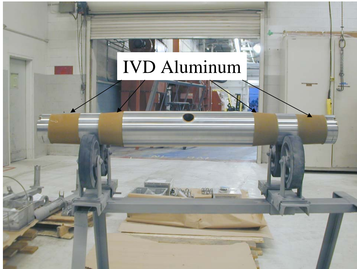
C-17 Axle After Conversion Coating
