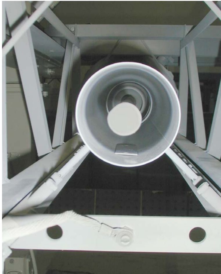
Sputter Probe Aligned In Center of Part
