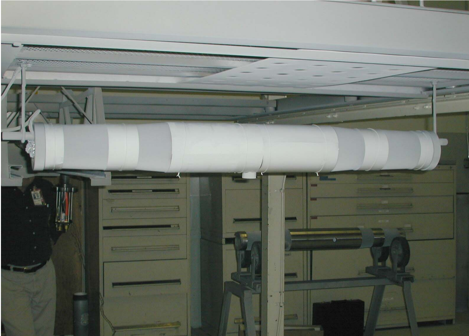
C-17 Axle After Sputter / IVD Aluminum Coating
