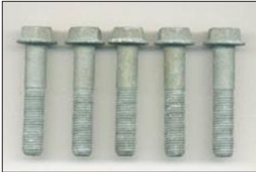
ASTM B117 Salt Spray 1000 hours
