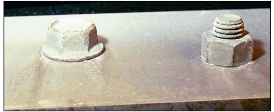
Magni 565 fasteners fastened into aluminum panel GM9540P - 120 cycles
