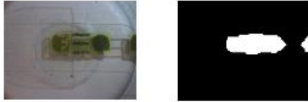
Figure 42: Comparison of an actual video frame and the same frame processed in MATLAB to compute the centroid of the robot in order to track its position over time.
