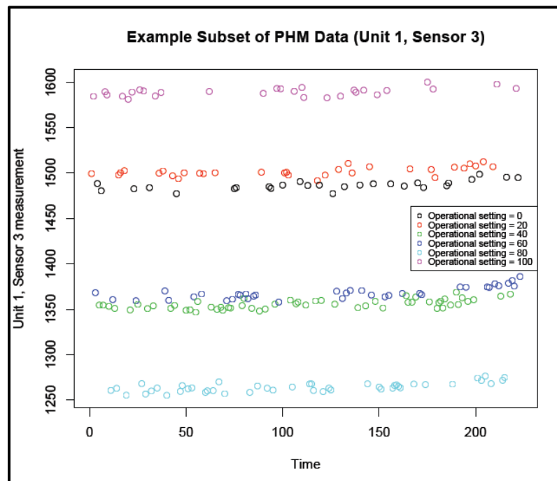
Figure 19: Subset of PHM data displaying various levels of normal operation corresponding to different control settings
