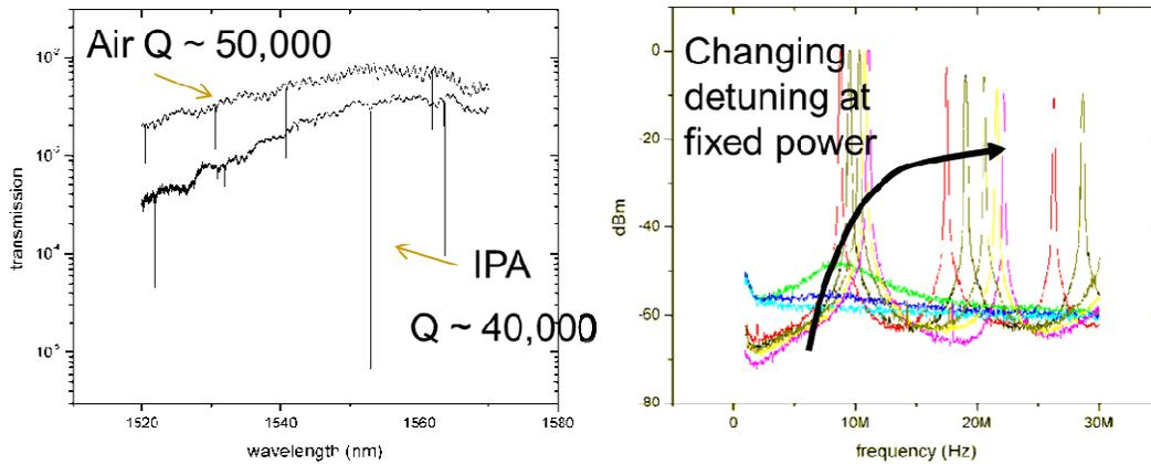
Figure 3. (a) Observed high Q optical resonances ( $Q \sim 50,000$ ) when optomechanical oscillator operated in air and in IPA at 1550nm. Since IPA is not absorbing at this wavelength, we did not find significant quality factor degradation when the device was submerged in IPA. (b) When immersed in IPA, the device displays spontaneous oscillations as a result of fluid-opto-mechanical interactions.
