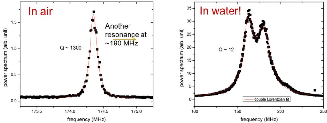
Figure 6. Mechanical resonances observed in air and in water. Although the quality factor is degraded when immersed in water (down to 12), the resonances are clearly observable with very high signal to noise ratio.
