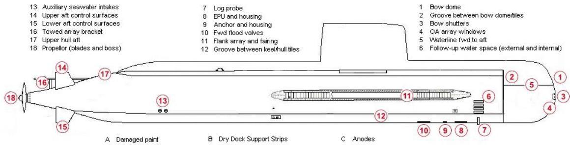
Figure 1. Collins Class submarine hull features (URS, 2006)
