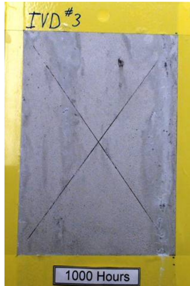
1000 Hours in ASTM B 117 (Scribed Corrosion Test) – Cold Spray Al on Steel (Left) and Cold Spray Al on Damaged IVD Al (Right)
