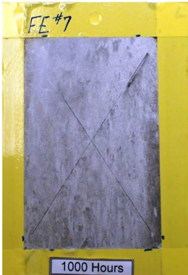
1000 Hours in ASTM B 117 (Scribed Corrosion Test) – Cold Spray Al on Steel (Left) and Cold Spray Al on Damaged IVD Al (Right)
