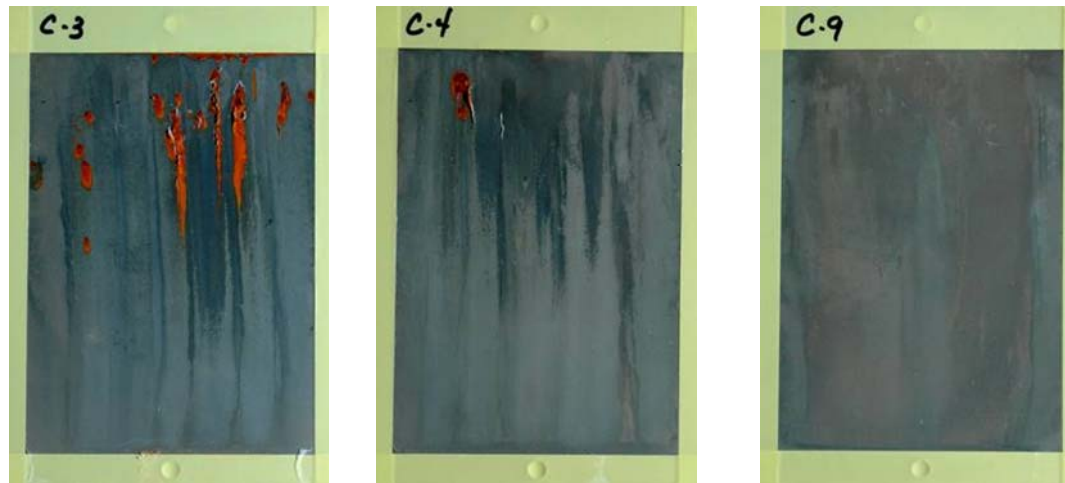
LHE Cadmium – 500 Hrs in ASTM B 117
