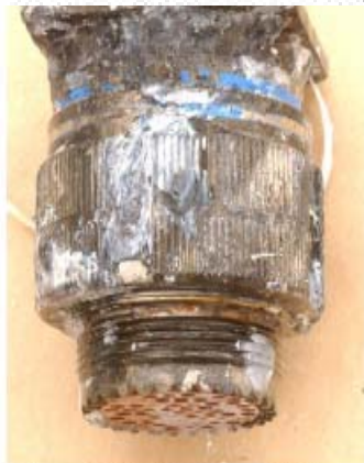
Figure 6.1.5 TTH after 336 hours in SO 2 -salt fog
