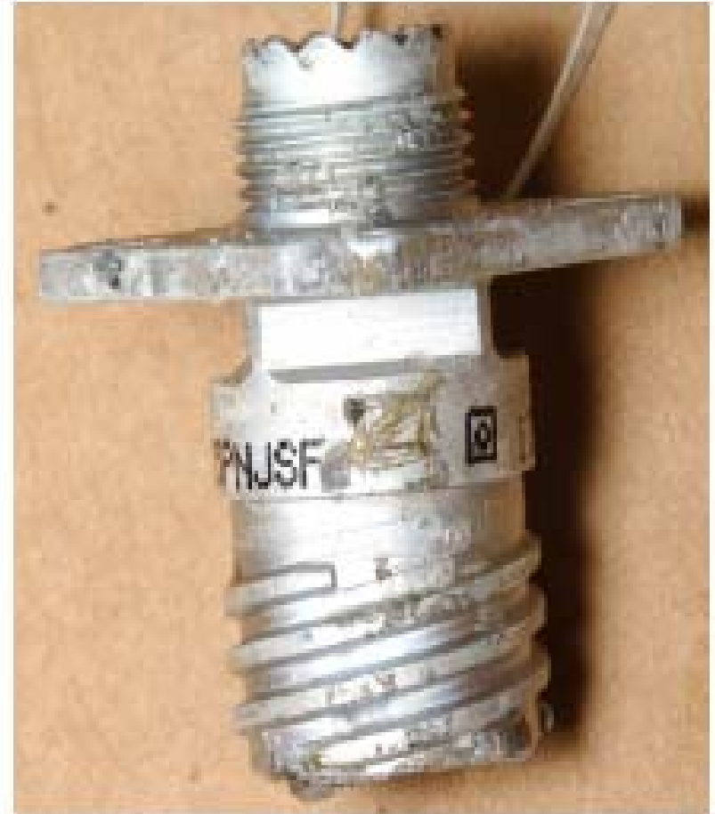
Figure 6.5.2 Cannon Alumiplate connector with clear coating after 338 hours in SO 2 -salt fog
