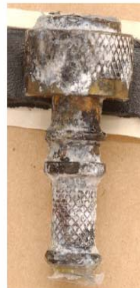
Figure 6.1.3 Bright Zn/Ni after 336 hours in SO 2 -salt fog
