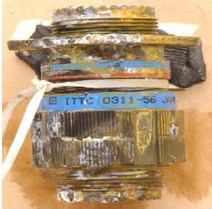
Figure 6.1.11 Ni/Cd connector after 336 hours in SO 2 -salt-fog
