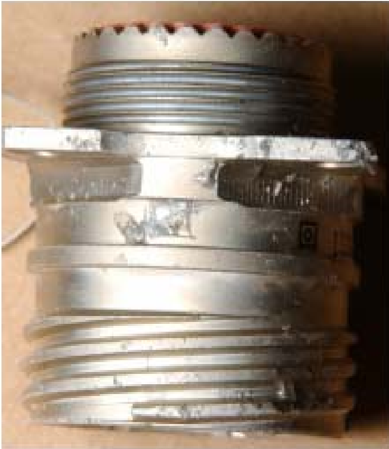
Figure 6.5.1 Cannon Alumiplate connector with chemfilm after 338 hours in SO 2 -salt fog
