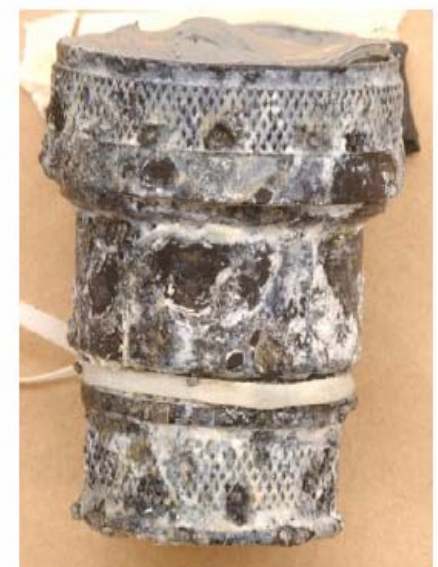
Figure 6.1.4 Dull Zn/Ni after 336 hours in SO 2 -salt fog
