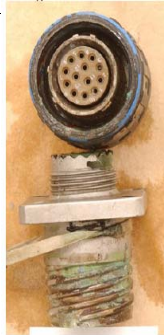
Figure 6.1.9 Dull Ni composite after 336 hours in SO 2 -salt fog
