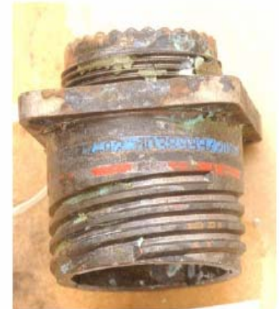
Figure 6.1.10 Bright Ni composite after 336 hours in SO 2 -salt fog
