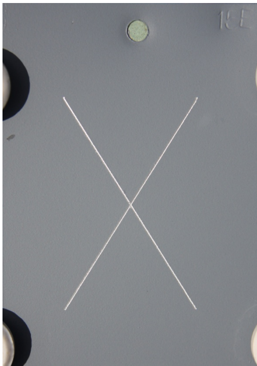
Topcoated Commercial Cr (VI) spray primer with Cr (VI) pretreatment
