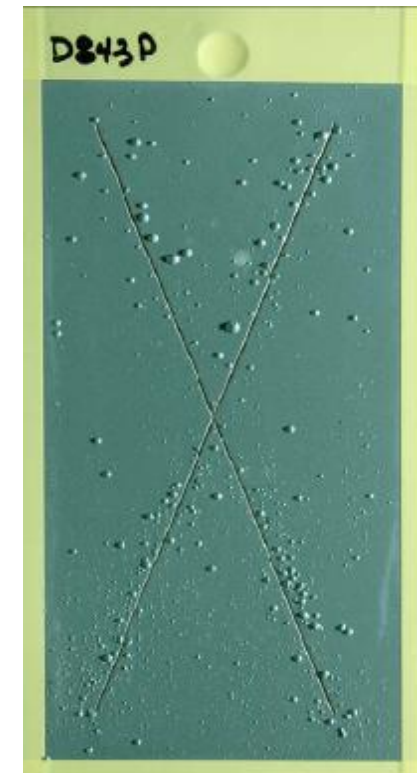
Commercial Cr (VI) spray primer with Cr-free pretreatment
