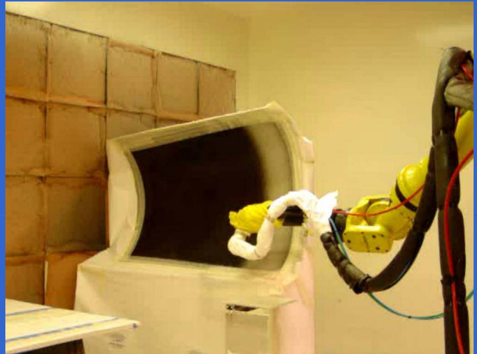
Robotic Spray System Spraying Contoured Mock-up Part
