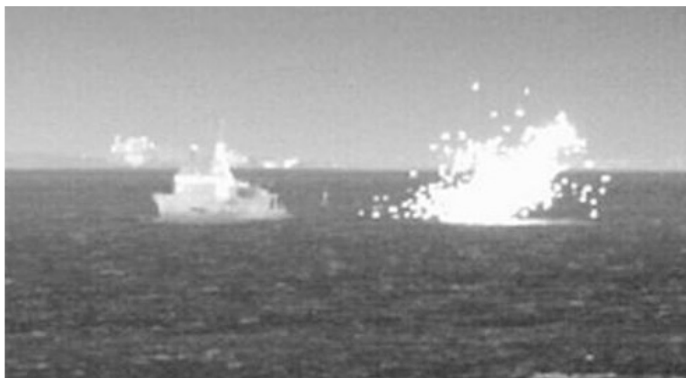
Figure 6: Short-Range IR Image of the ROSY Decoy.
