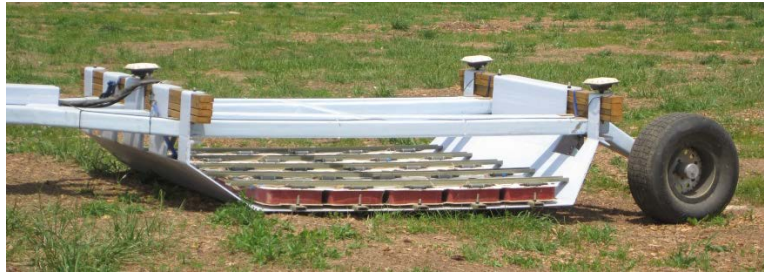
Figure 5-2 – Sensor array mounted on the MTADS EMI sensor platform.
