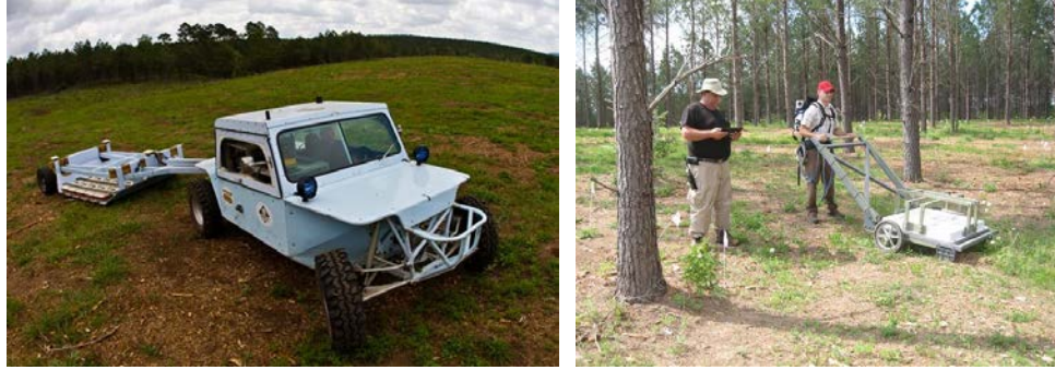
Figure 4-3 – 5x5 Array (left) and MP System (right) collecting data at the fSpAR demonstration site
