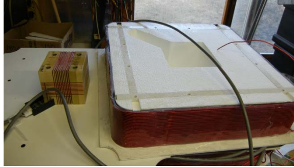
Figure 2-2 – Individual TEMTADS/3D EMI sensor with 3-axis receiver under construction.
