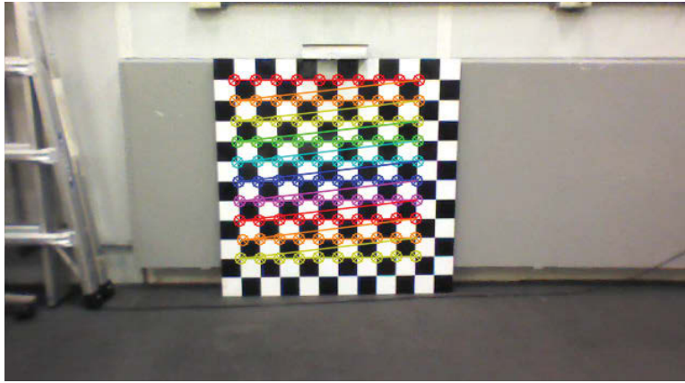
Figure 3.6: Automatic Camera Calibration. The ROS camera calibration package automates camera calibration by recognizing a calibration pattern.
