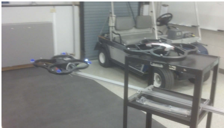
Figure 4.1: Testing Equipment. The equipment shown was used to keep the lead vehicle with illuminated targets in view of the trailing vehicle during tests.
