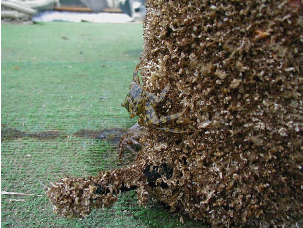
Figure 4.23 Close-up of Fouled Spill Sentry Buoy.
