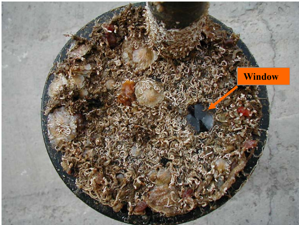
Figure 4.24 Fouling around Optical Window.
