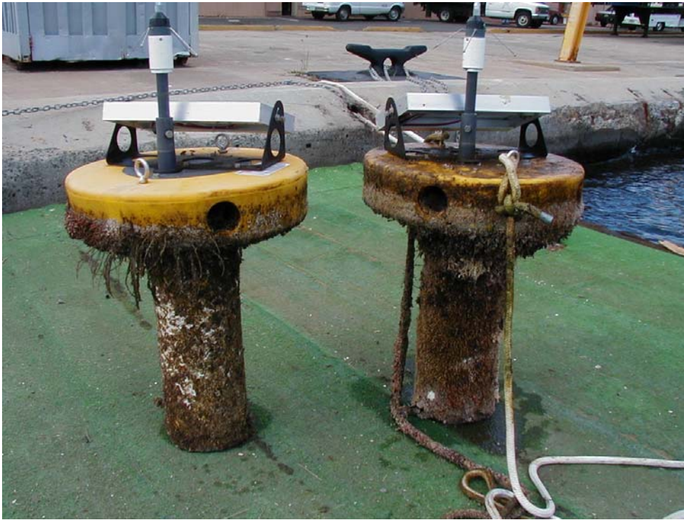
Figure 4.22 Sensor Fouling at Pearl Harbor, HI.
