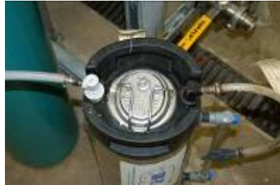
Culture Keg with Quick Disconnects Pressurized with N 2
