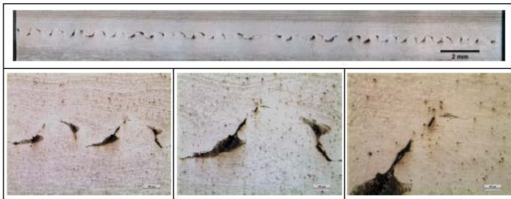
Figure 11: Macrographs and micrograph of plate 7 TWIP (2.6) + TWIP (2.6). Top scale bar is 2 mm.
