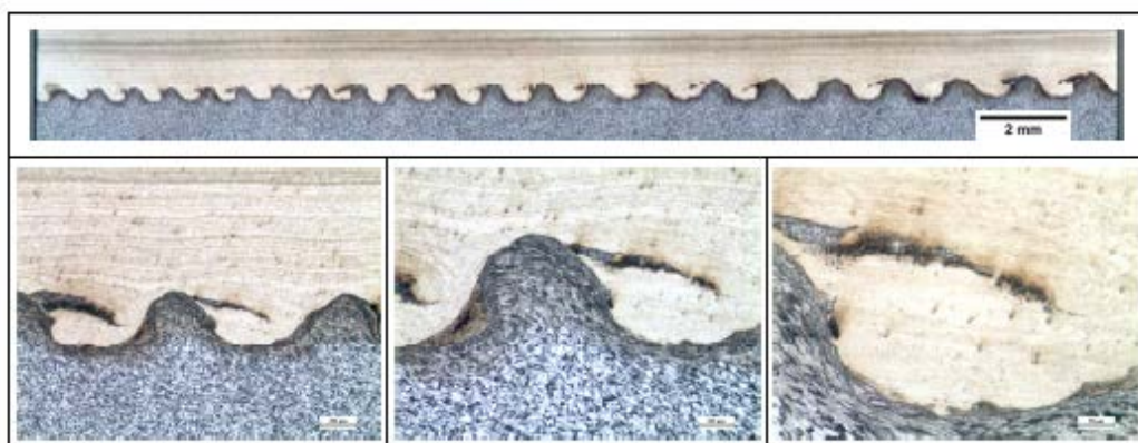
Figure 6: Macrographs and micrograph of plate 2 G350(8.5) + TWIP (2.6). Top scale bar is 2 mm.
