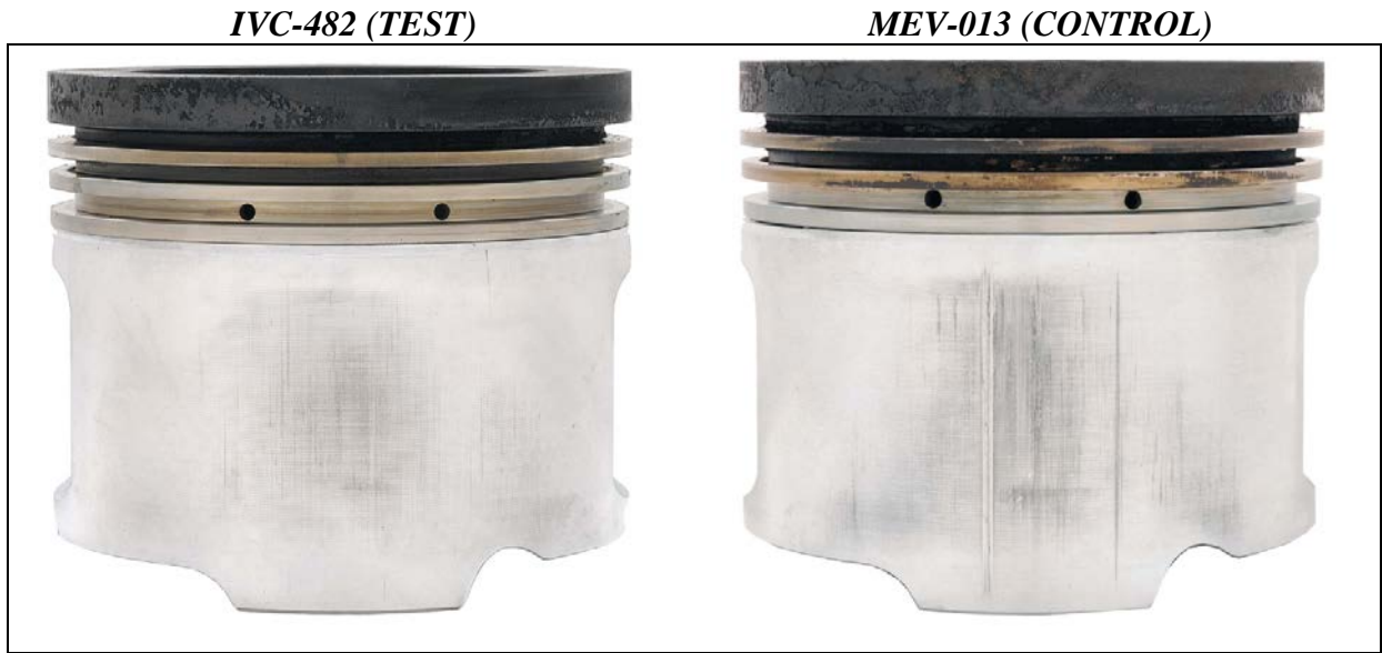
Figure 6. Thrust Side, Piston Skirt “Worst”, TEST: #1, CONTROL: #4
