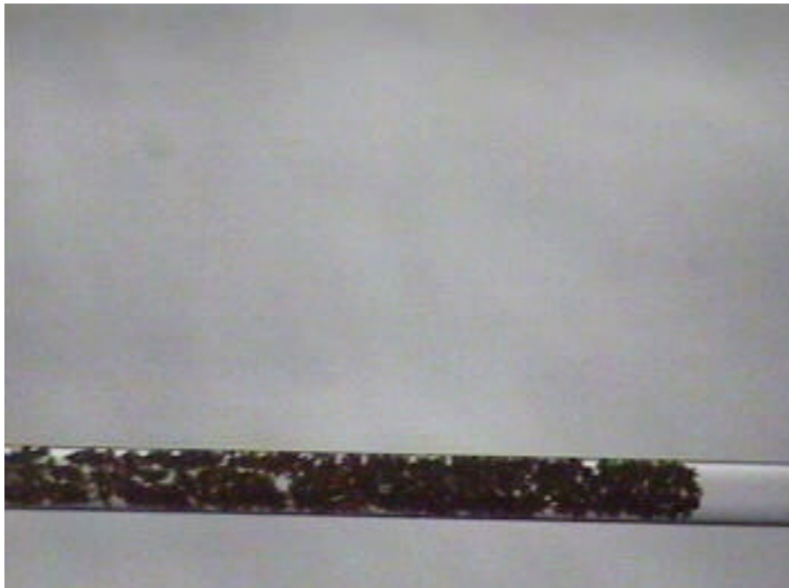
Figure 18. Photo of SPE Column Packed with C18 Coated Paramagnetic Beads
