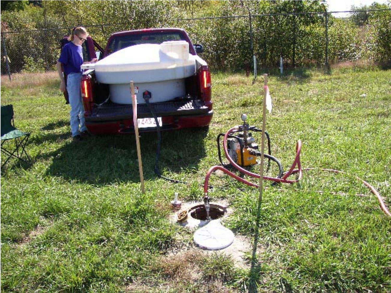
**Figure 2-4. Reagent Mixing and Injection System**
