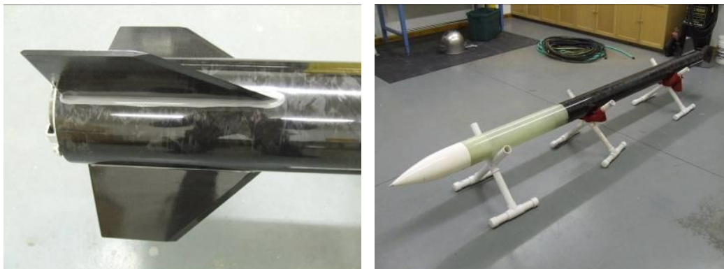
Figure 31 - Outer Surface Clear Coated, Buffed and Waxed
