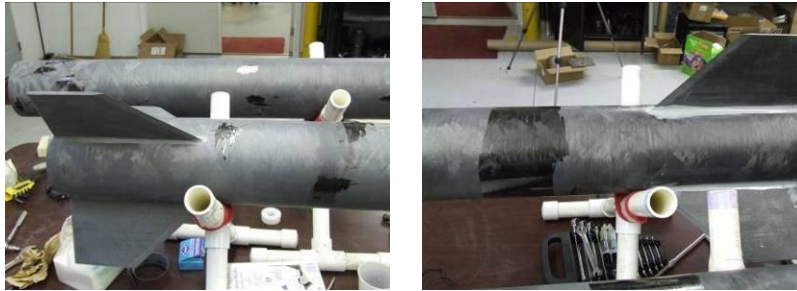
Figure 29 – The joint and small voids on the outside surface of the airframe tube were filled with epoxy and sanded flush and smooth.
