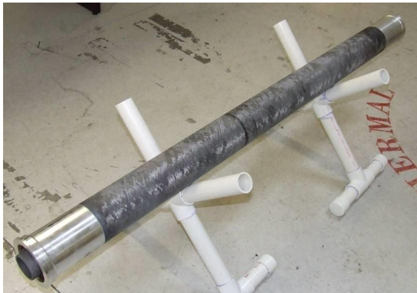
Figure 122 – Carbon Fiber/Epoxy Motor Casing
