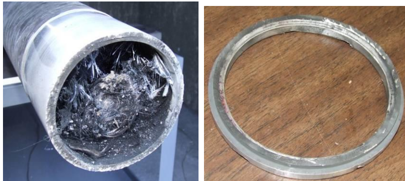
Figure 8 – Shear Failure of End Cap
