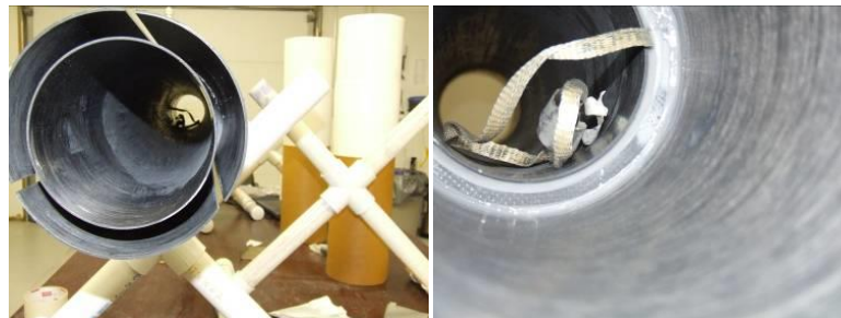
Figure 25 – The centering tube is permanently attached to the inside of the airframe tube using centering rings and urethane adhesive.
