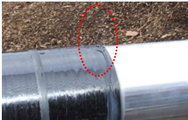
Figure 17 – Leak detected in the motor casing at 750 psi.
