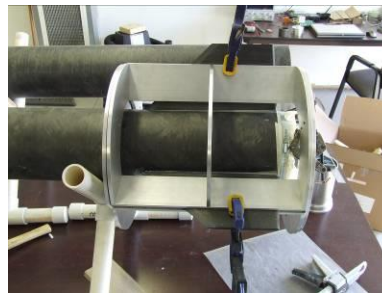
Figure 27 – The fin fixture was used to position the fins while adhesive cured.
