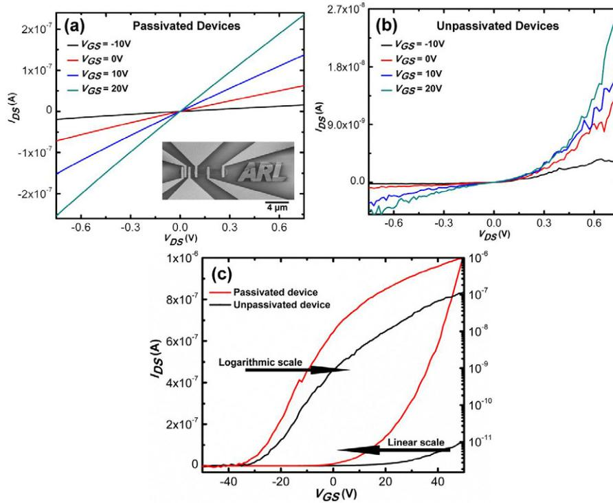
**Figure 1.**  $I_{DS}$ – $V_{DS}$  plot at 300 K for MoS<sub>2</sub> FET (a) before and (b) after etching of the top passivation. All the  $I$ – $V$  curves were taken at constant drain–source voltage ( $V_{DS} = 0.5$  V). The inset in (a) shows an SEM micrograph of a typical device. (c)  $I_{DS}$ – $V_{GS}$  plot of the passivated and unpassivated devices plotted in both linear and logarithmic–linear scales at 300 K.
