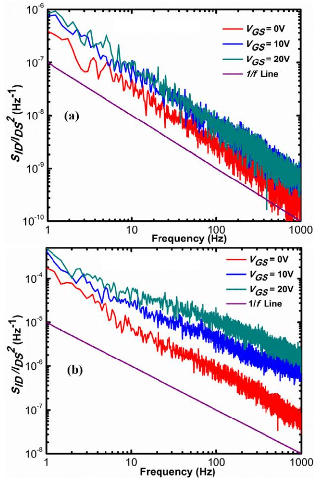
**Figure 3.** Room temperature ( $T = 300$  K) normalized PSD of the drain current for (a) passivated and (b) unpassivated (after etching of the top passivation) devices at different  $V_{GS}$ . A  $1/f$  trend line is shown for comparison. All the readings were taken at a constant drain–source voltage ( $V_{DS} = 0.5$  V).
