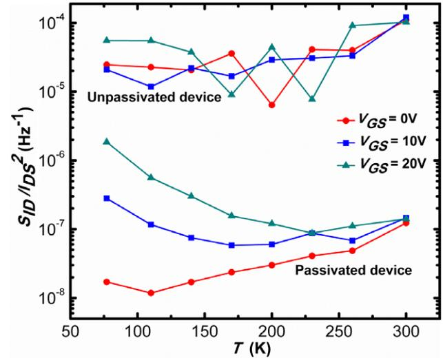
**Figure 6.** Temperature-dependent (77–300 K) normalized PSD of the drain current noise at  $f = 10$  Hz at different temperatures for passivated and unpassivated (after etching of the top passivation) devices. All the readings were taken at constant drain–source voltage ( $V_{DS} = 0.5$  V).
