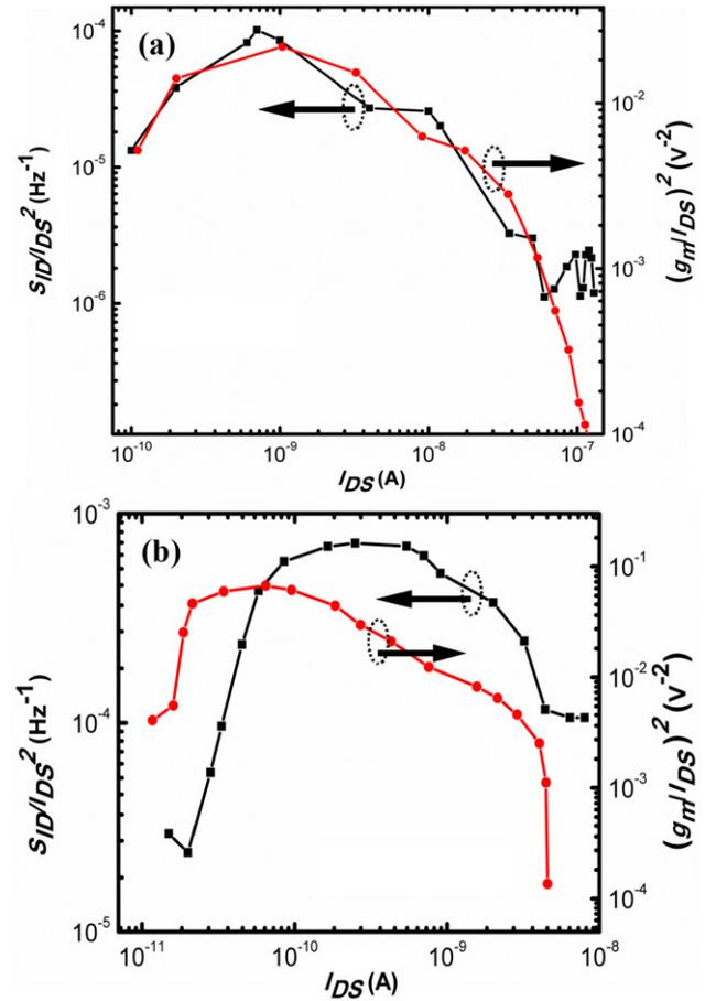
**Figure 4.** Comparison of normalized PSD of the drain current at  $f = 1 \text{ Hz}$  and  $(g_m/I_{\text{DS}})^2$  at different  $I_{\text{DS}}$  for passivated and unpassivated (after etching of the top passivation) devices in (a) and (b), respectively. All the readings were taken at a constant drain–source voltage ( $V_{\text{DS}} = 0.5 \text{ V}$ ).
