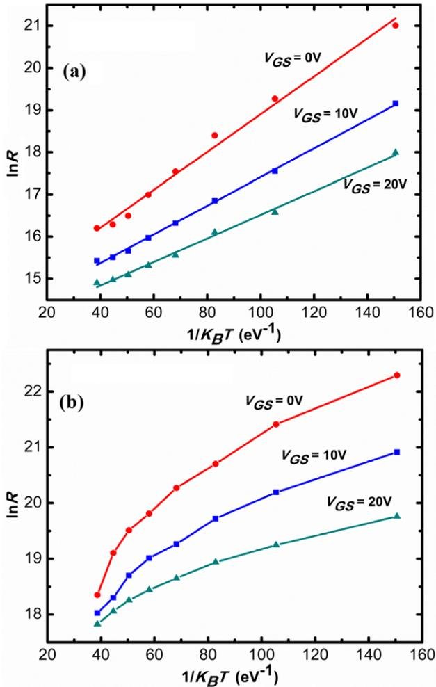
**Figure 2.** Arrhenius plot of the drain–source resistance of the passivated and unpassivated (after etching of the top passivation) FETs at three different gate biases is shown in (a) and (b), respectively. Temperature is in the range of 77–300 K. All the readings were taken at a constant drain–source voltage ( $V_{DS} = 0.5$  V).
