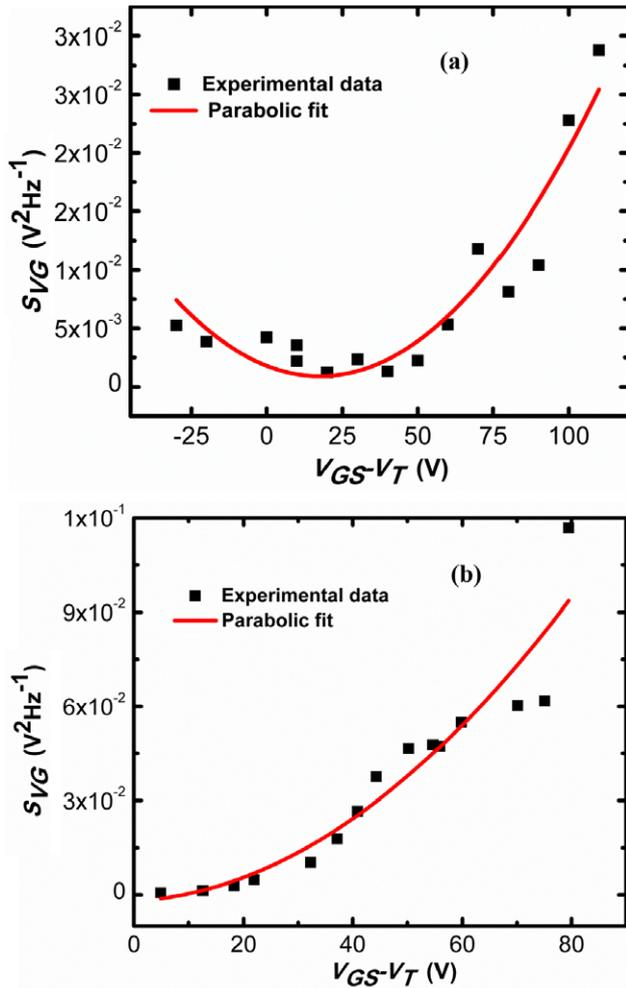
**Figure 5.** The experimental input gate-referred PSD voltage obtained at different  $V_{GS}$  values for (a) passivated and (b) unpassivated (after etching of the top passivation) devices. Parabolic fit to the measured data points is also shown. All the readings were taken at a constant drain–source voltage ( $V_{DS} = 0.5$  V).
