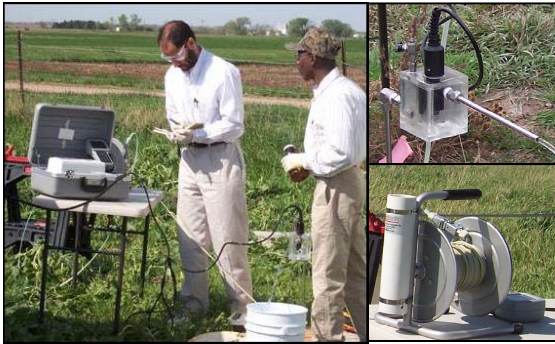
Figure 21. Sampling extraction well and sampling equipment.
