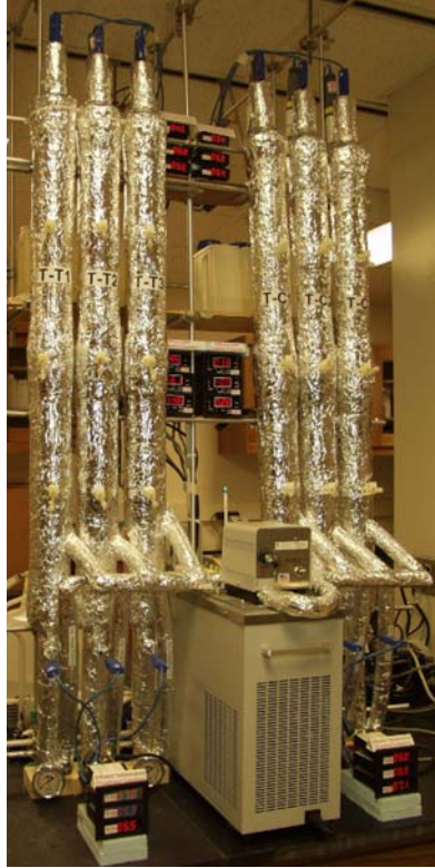
Figure 2. Experimental column setup for temperature study
