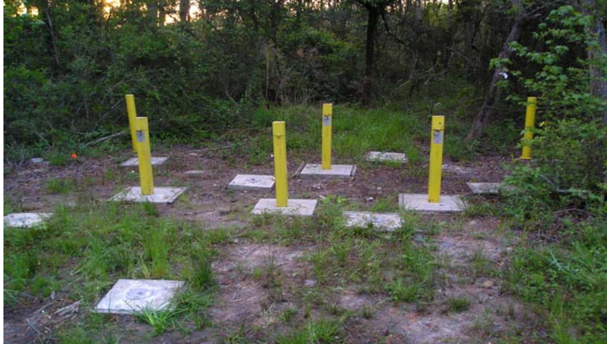
Figure 5-7. Photograph of Test Cell Showing Typical Monitor and Injection Wells (Three monitor wells and one soil gas monitoring point have above ground protective casings; injection wells are finished with flush-mount manhole covers. Two bollards are located on the left and right at the rear corners of the cell.)
