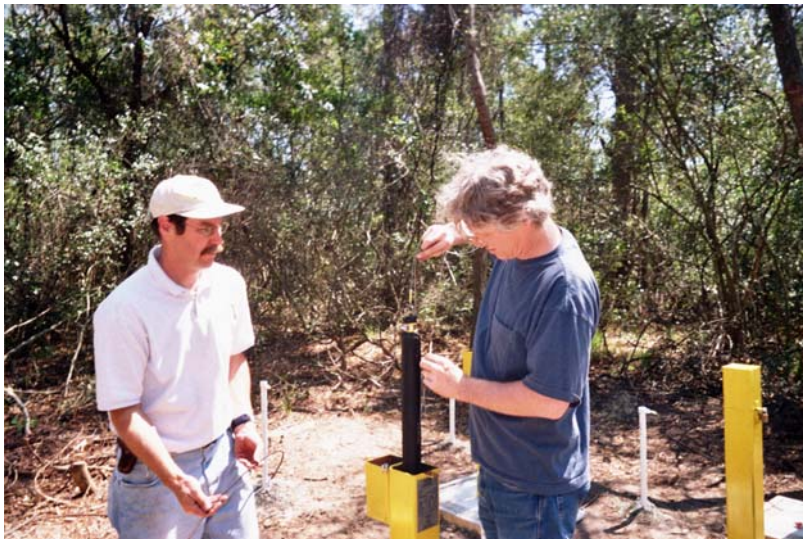
Figure 7-17. Photograph of Installing a Mass Flux Canister into a Monitor Well in the Test Cell
