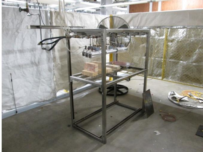
Figure 7 Quartz Lamp Fixture
