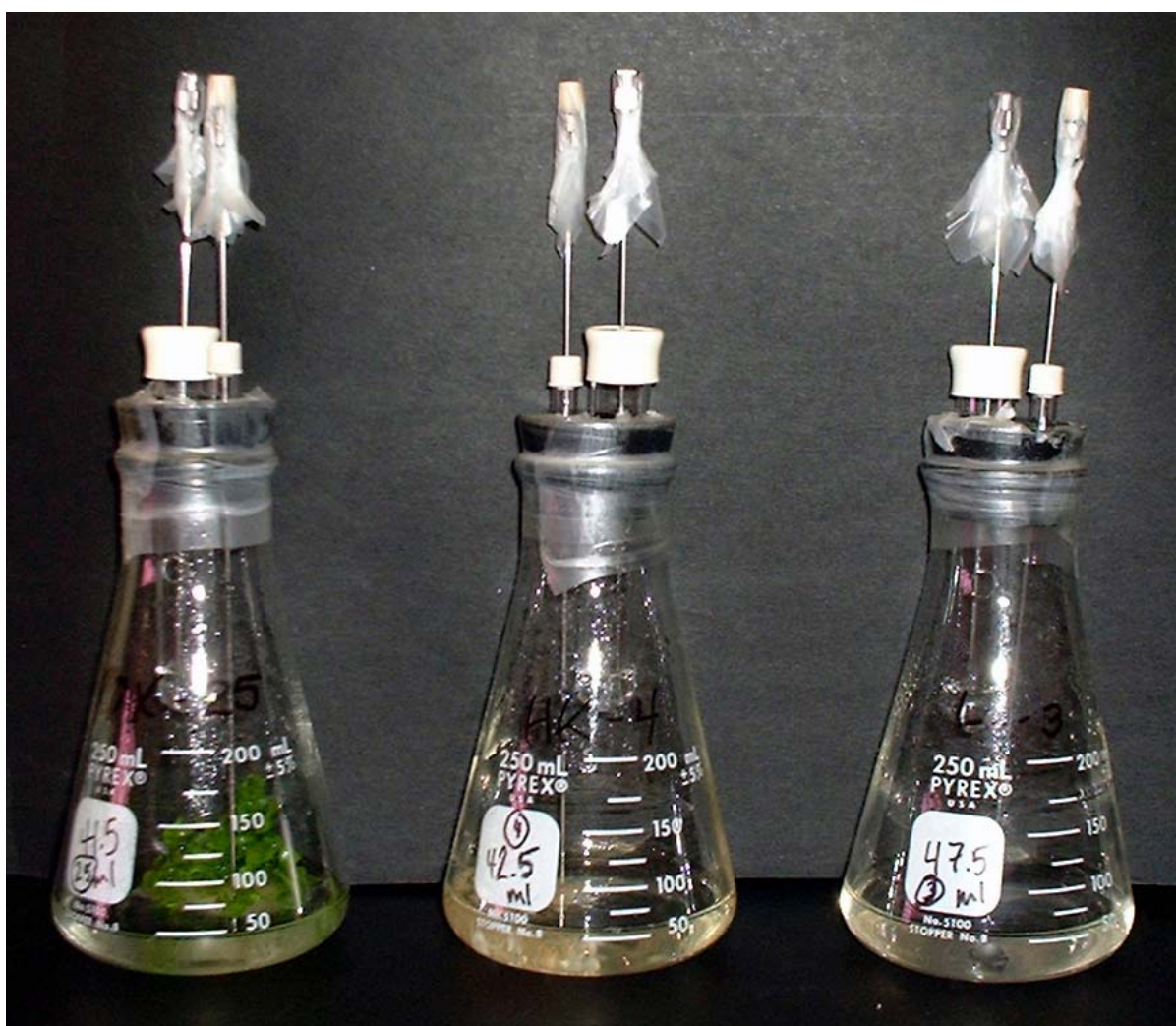
Figure 3.3. A sample flask, a heat-killed control flask and a light control flask. Figure was taken when plants were 19 days old and 9 days after RDX was added to the flasks.
