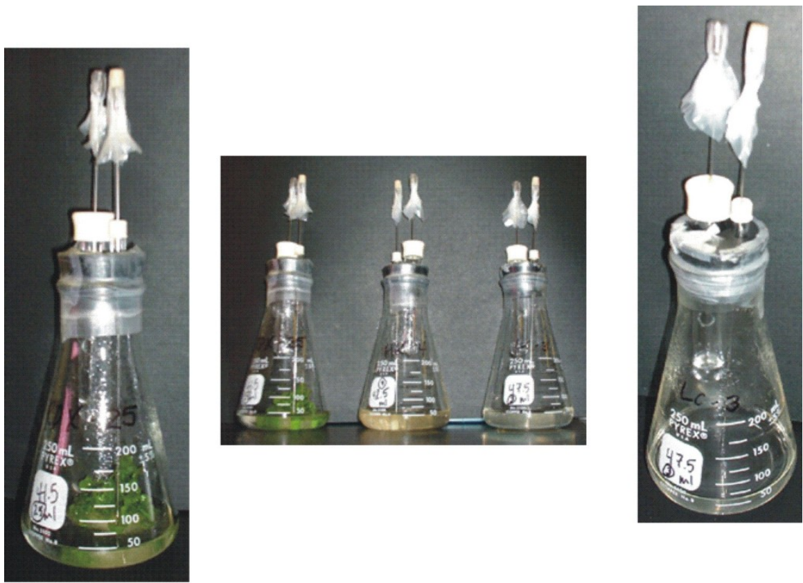
Figure 25A: Experimental set up showing the various ports in the sterile flasks to draw out samples and trap carbon dioxide.
