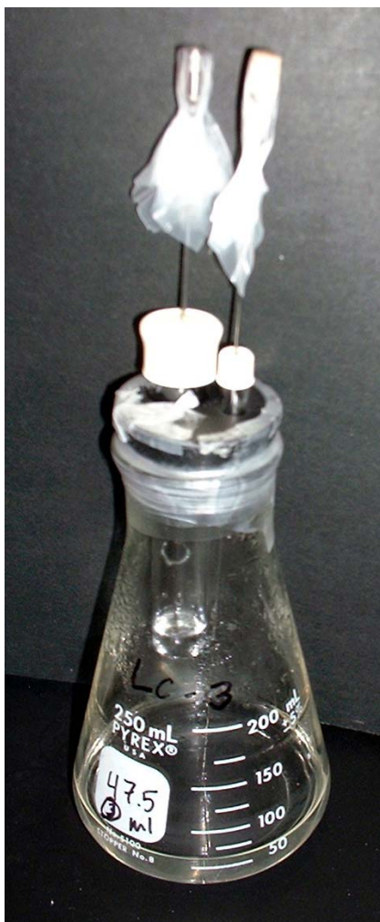
Figure 3.2. A flask used in the experiment. The rubber stopper apparatus sealed with Parafilm can be seen. Potassium hydroxide is also visible in the test tube.
