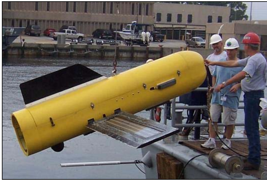
Figure 3 BOSS-160 vehicle with aft mounted RTG
