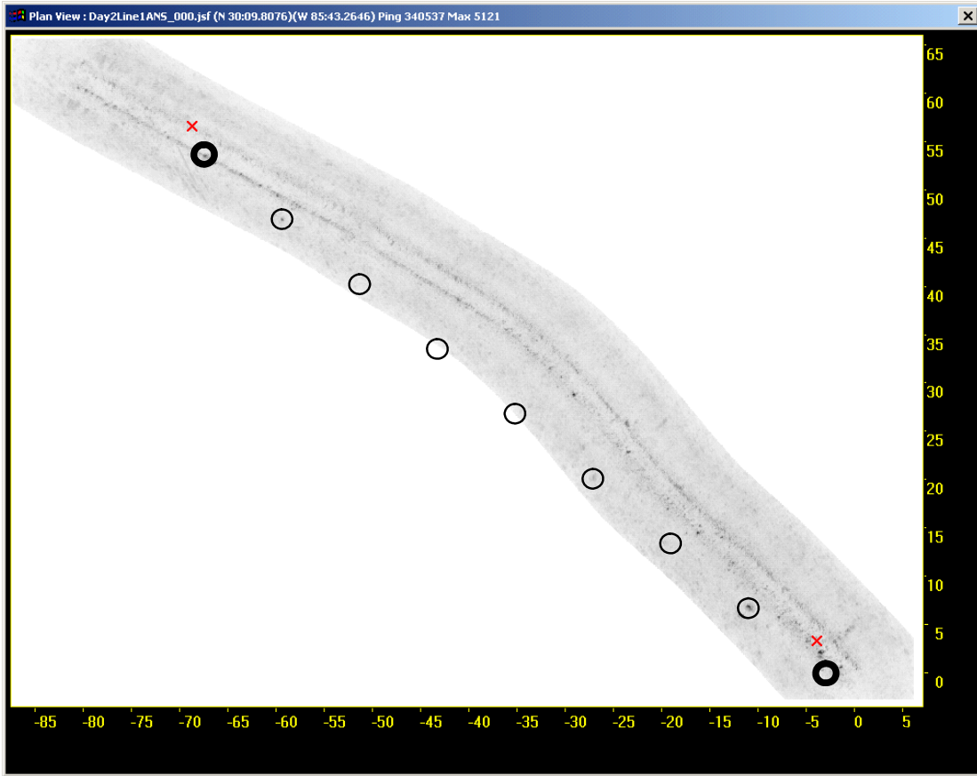
Figure B - 8. Multi-aspect image of trackline Day2Line1ANS collected on 19 October 2006 at sand site with target overlay
