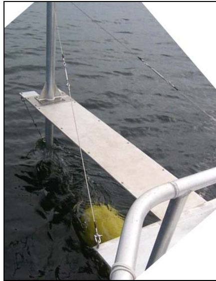
Figure 10 Photo of bow mounted pole used to tow the BOSS-160 sonar at a depth of approximately 1 meter during transit.
