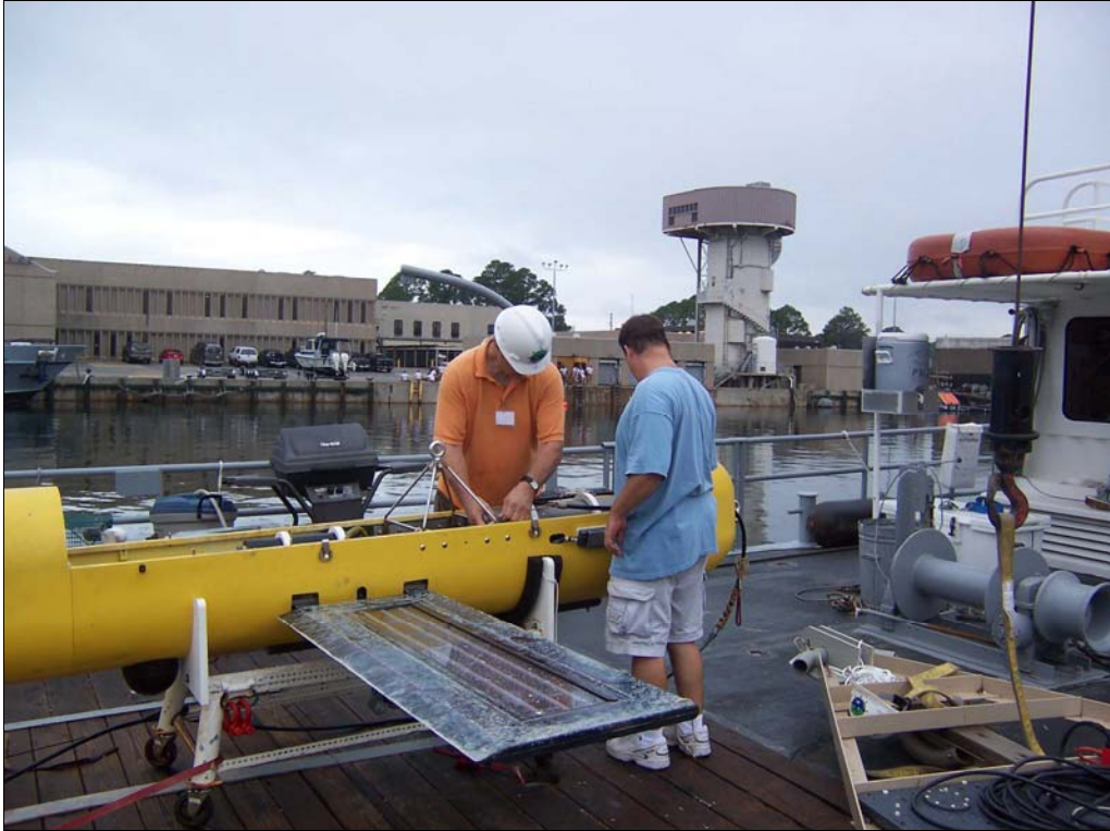
Figure 18 RTG sensor is installed in the BOSS towed vehicle during Phase I pretest operations
