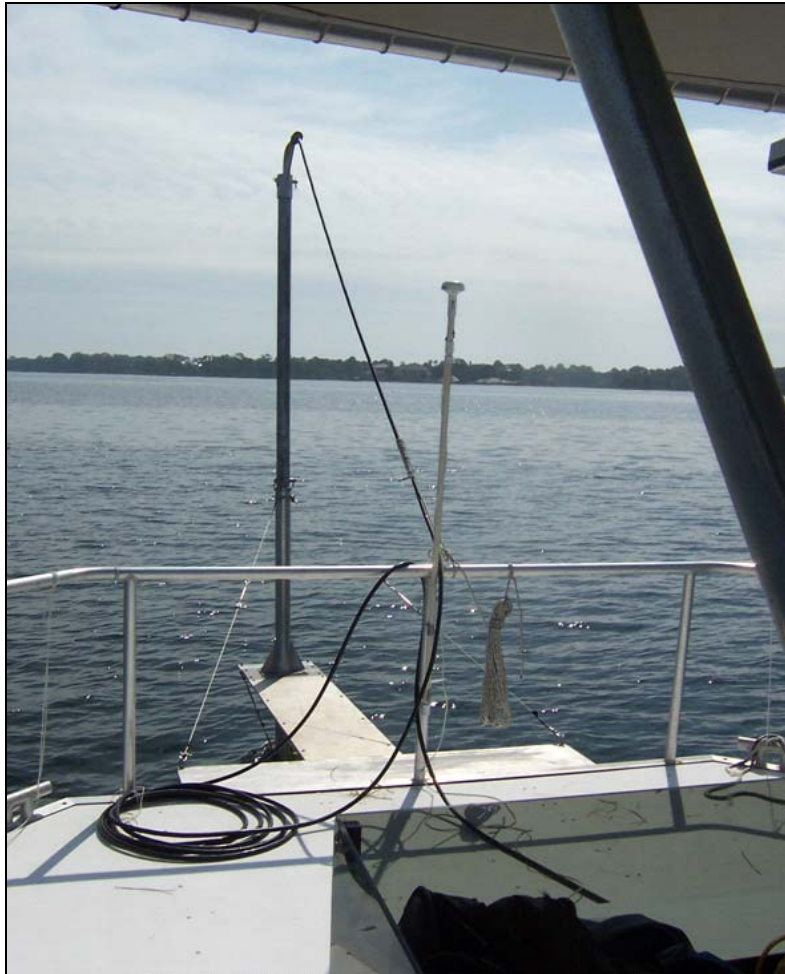
Figure 22 Photo of WAAS GPS antennae mounted directly above the sonar vehicle being towed from the pole. The GPS was aligned to a point above the center of the two sonar vehicle wings.
