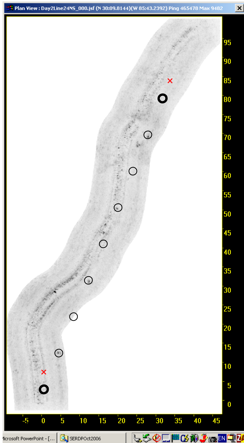
Figure B - 16. Multi-aspect image of trackline Day2Line24NS collected on 19 October 2006 at sand site with target overlay
