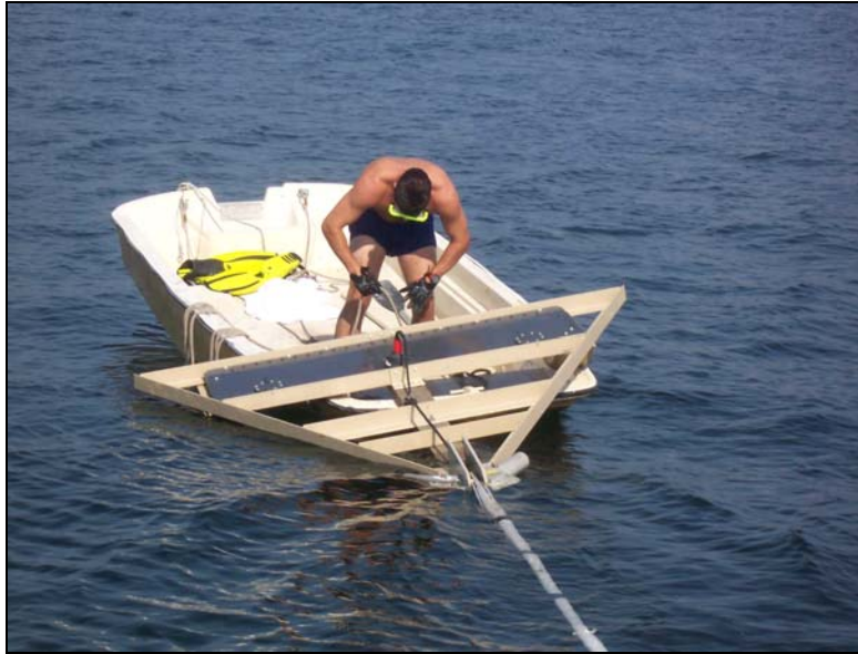
Figure 20 GEM-3 array mounted on whaler for transit to test area
