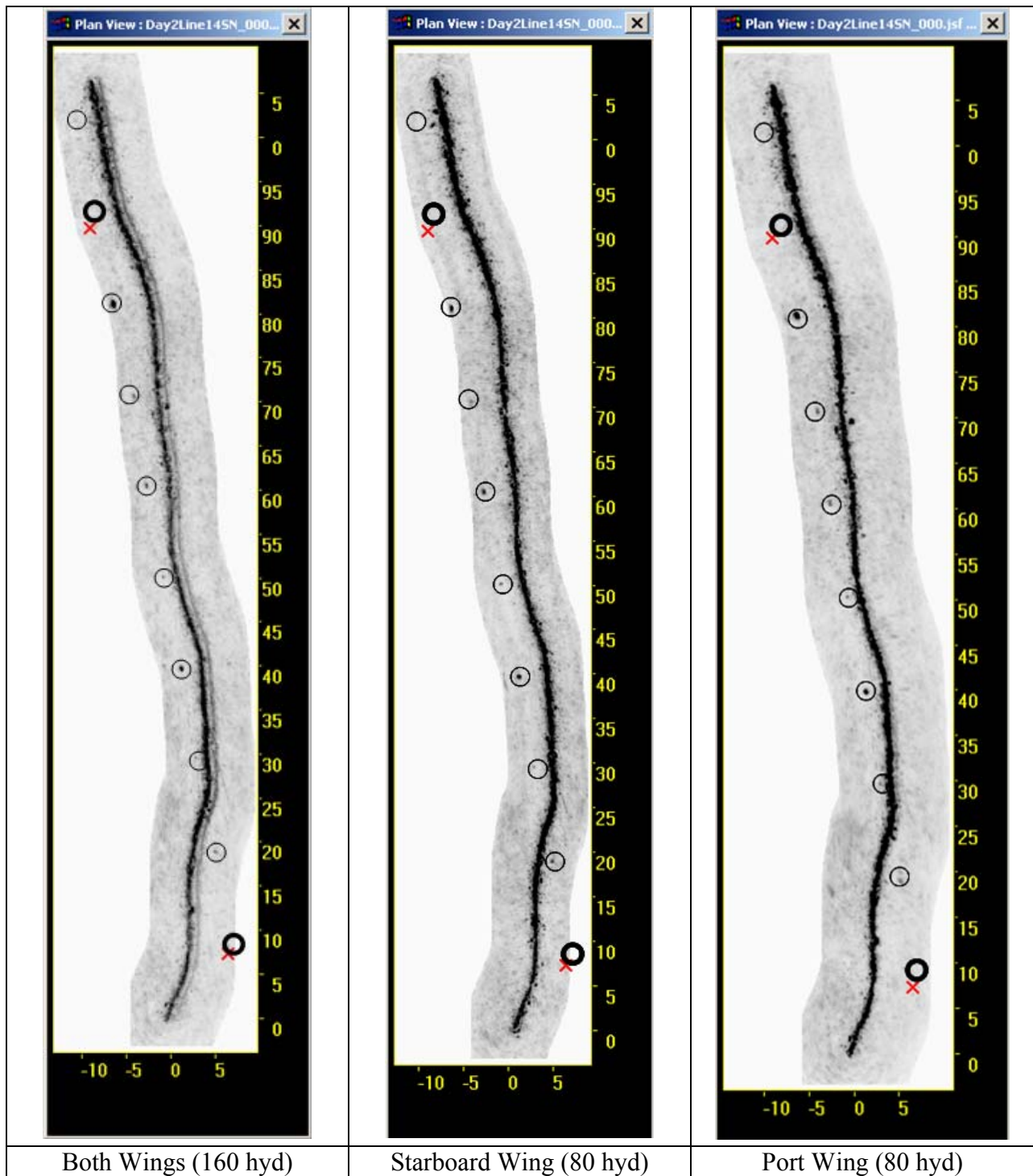
Figure 29 Comparison of images generated with all hydrophone channels (both wings), starboard wing channels and port wing channels. (Run # Day2Line14SN)
