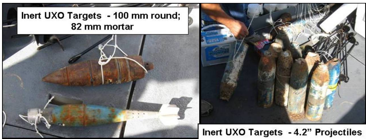
Figure 71 Phase II inert UXO Targets
