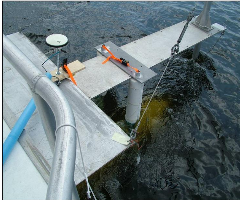
Figure 69 RTK GPS antenna and vertical BOSS vehicle harness in the Phase II configuration NovaTel RT2 equipment was used to perform the RTK GPS measurements. The shore-based reference NovaTel RT2 unit was located on the roof of an NSWC PC building ~ 1.5 kilometers from the shallow water test site.
