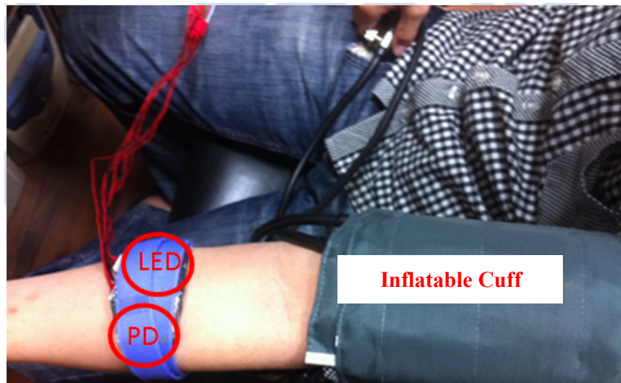
Figure 3. Experimental setup of an inflatable cuff and the NIRS probe.
