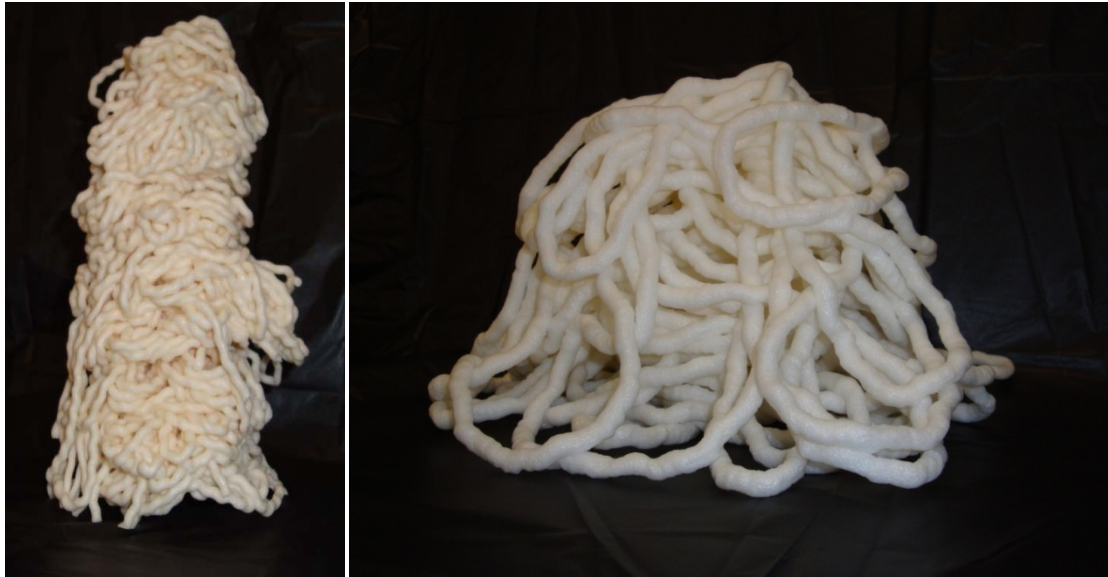
Figure 14: Initial foam strands (left) and improved foam strands (right)
