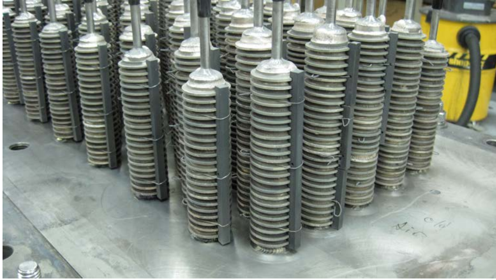
Figure 6- 4 Water Side Heat Pipes with Residue after First Furnace Run
