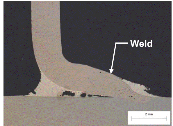
Figure 28 - Assembly #4 Braze Joint Voids with Porosity in Adjacent Weld
