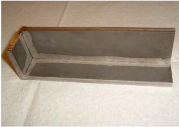
Ti Alloy T-Joint with Blind Corner Cleaned with Thermionic Cleaning
