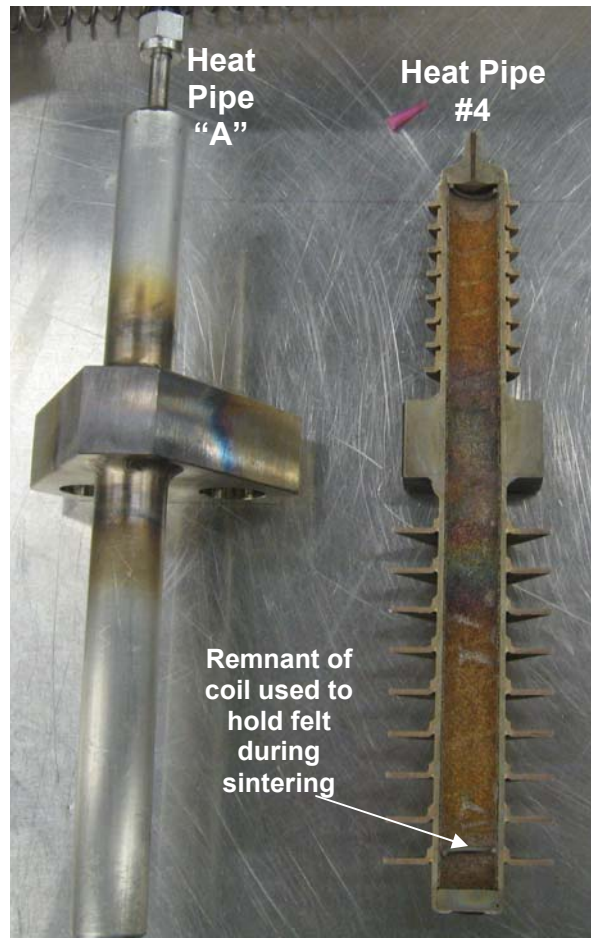
Figure 12 Heat Pipes #4 and “A”
