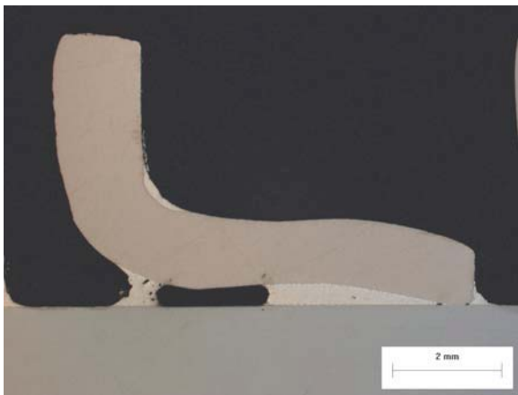
Figure 26 - Assembly #2 Braze Joint Voids with Bowed Fin Leg
