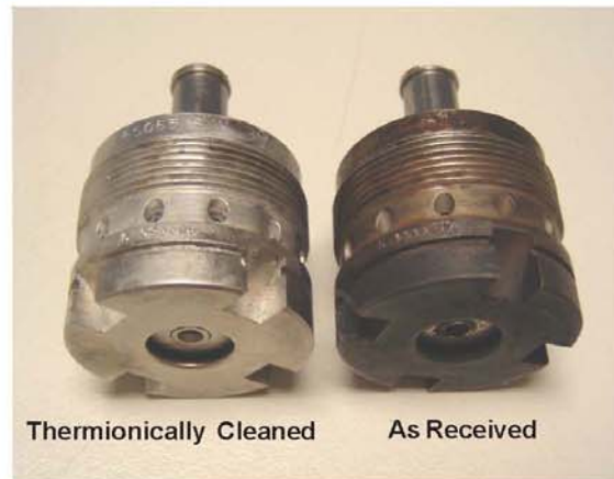
Gas Turbine Engine Fuel Nozzles
