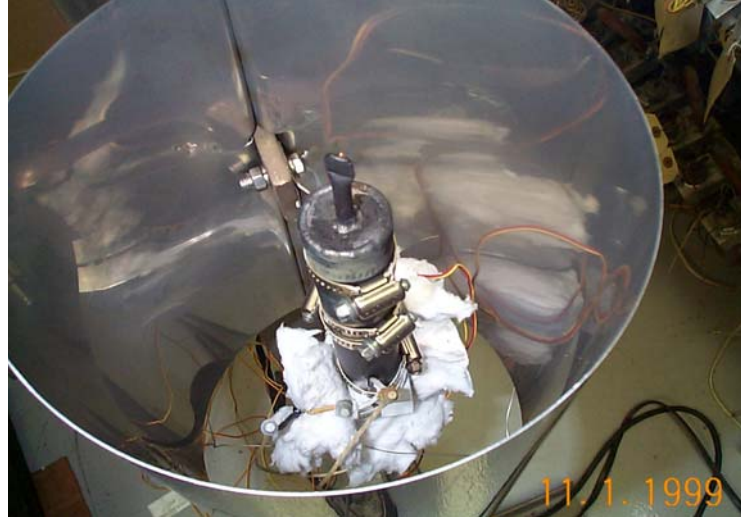
Figure C3. HP#748 on High Temp. Life Test
