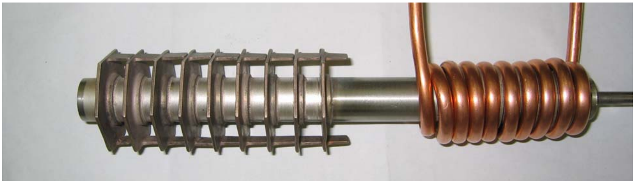
Figure 5 HP#2 Showing Water Cooling Coil
