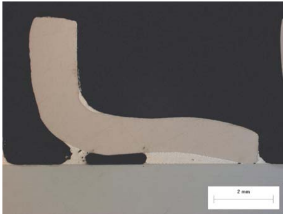
Figure 26 - Assembly #2 Braze Joint Voids with Bowed Fin Leg
