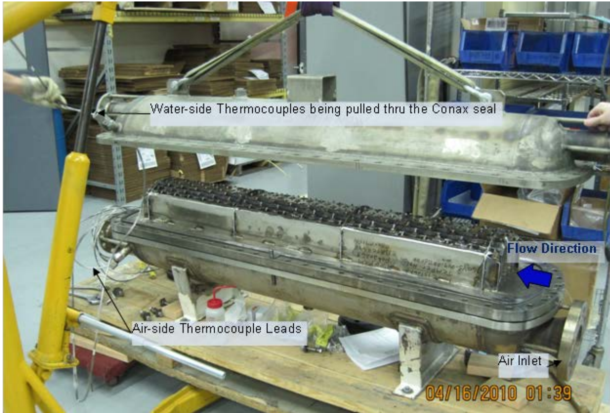
Figure 7- 2 Thermocouples being pulled thru Conax seal on Water Side Shell
