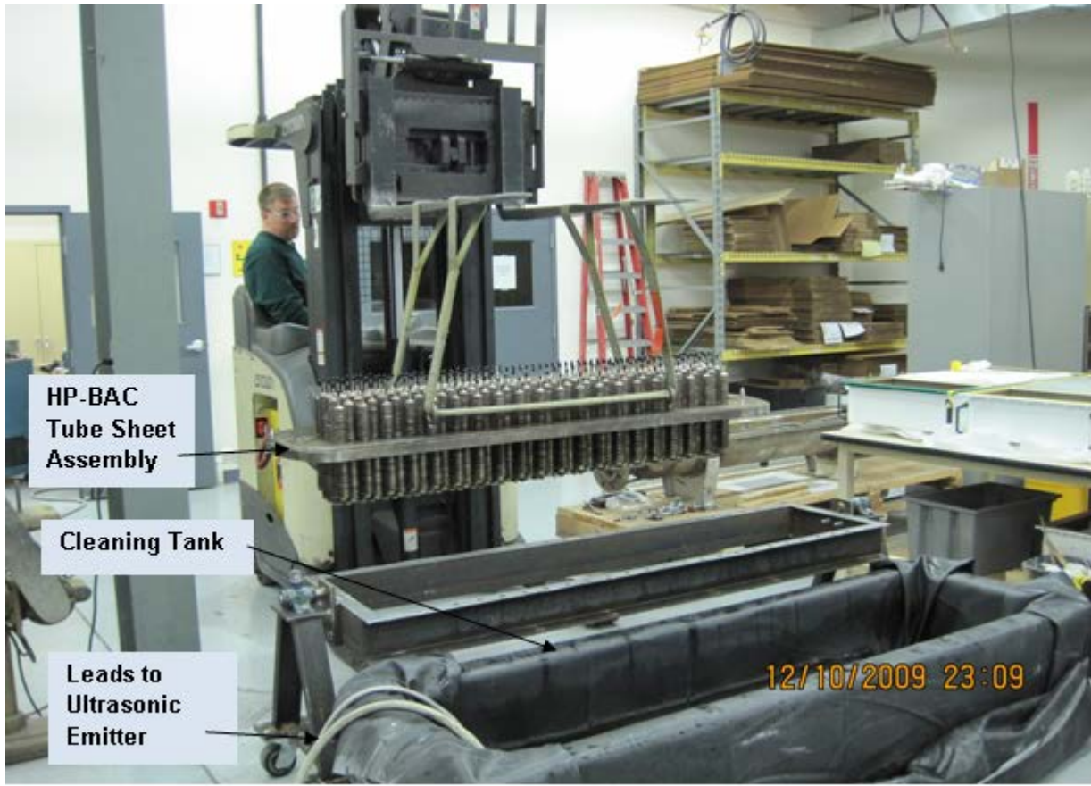
Figure 6- 6 HP-BAC Tube Sheet Being Immersed in Ultrasonic Cleaning Tank
