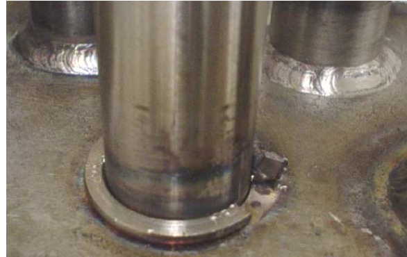
Figure 16 - ACT Consumable Insert Weld with Melt-Back
