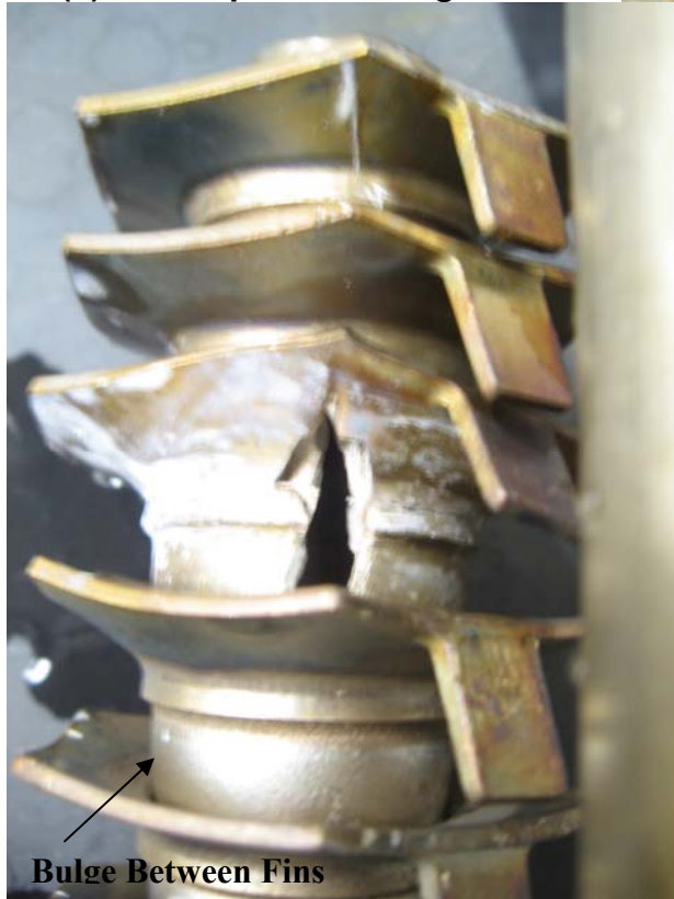
(c) Closeup of burst region
