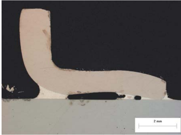
Figure 25 - Assembly #1 Braze Joint Voids with Bowed Fin Leg
