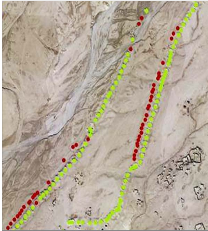
Figure 4.16: Chahs mapped within a portion of the lower study basin, where open and presumably viable chahs are indicated in green and those no longer open shafts in red. The parallel pattern of red to green symbols suggests bypassing of failed system segments.
