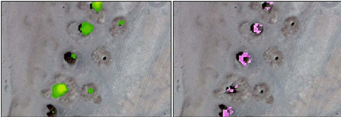
Figure 4.13. LiDAR-enhanced orthophotography. (L) Green-yellow color represents the last return, i.e., the open access shafts, and (R) purple represents the first return, i.e., crowns of tree growing within chahs.
