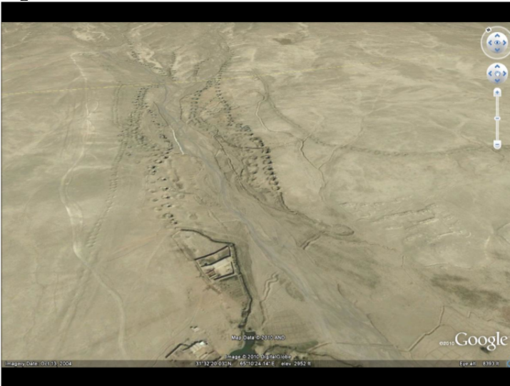
Figure 3.2: Enhanced Google Earth image of a karez, showing the vertical access shafts (chahs) and outflow channel leading to irrigated farms.
