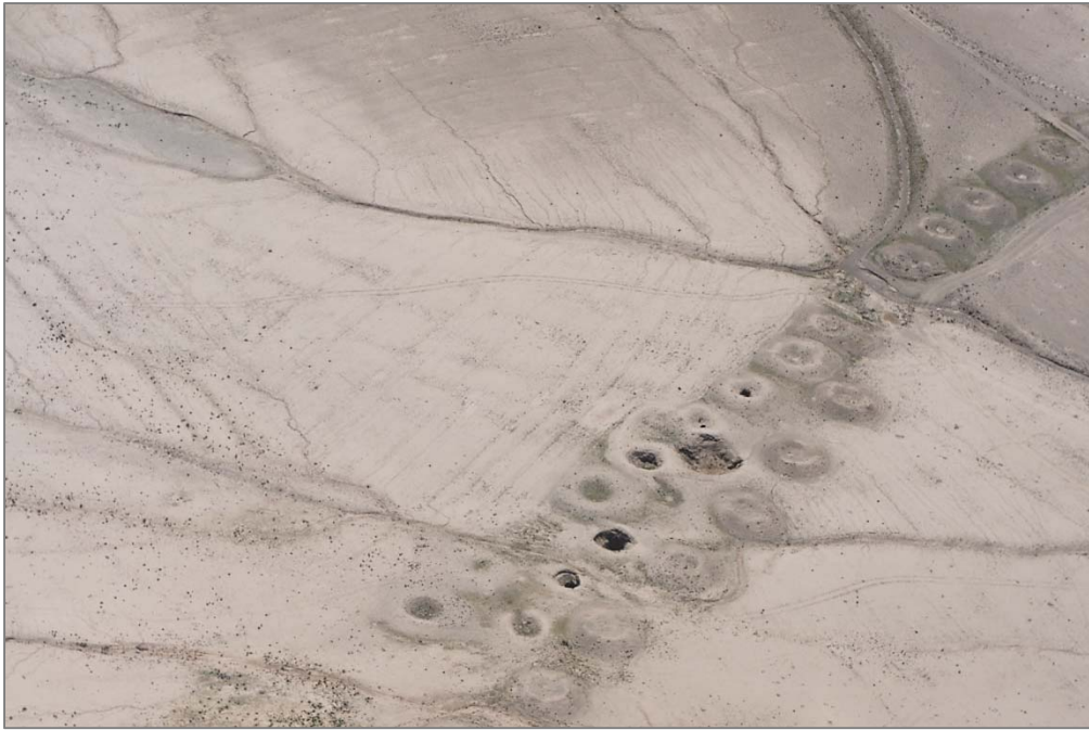
Figure 4.9: Segment of a karez where three generations of chahs indicated repeated failures of the conduit, requiring the lateral displacement of the system to by-pass the unusable portion. Note also that the surface drainage is at a near right angle to the karez alignment, which is not unusual given the relative independence of the surface water system from the ground-water system. (Image by W. Steele)
