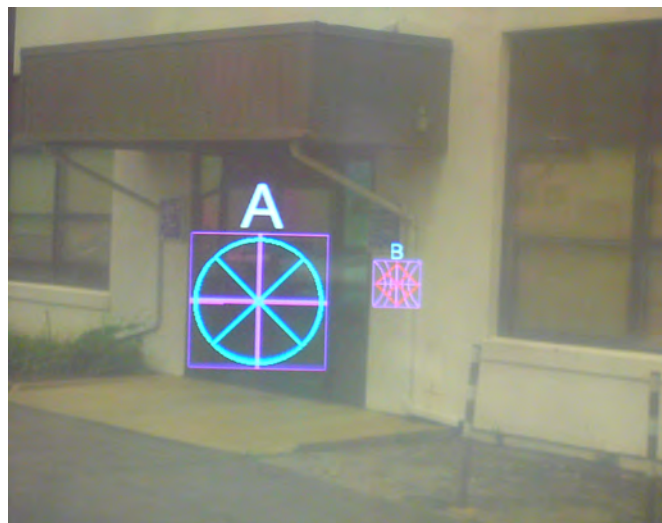
Fig. 10 The Virtual wall aimed to provide the cues of the Edge map, but with a less-cluttered and computationally less-demanding representation.
