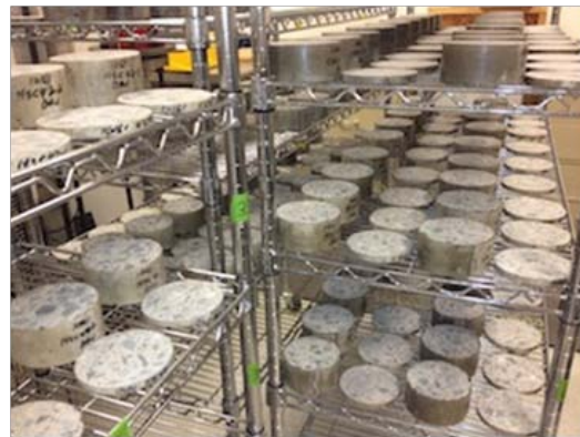
Figure 14-2. Moisture Transport Coefficient Drying Test (Photo by Tourney Consulting)
