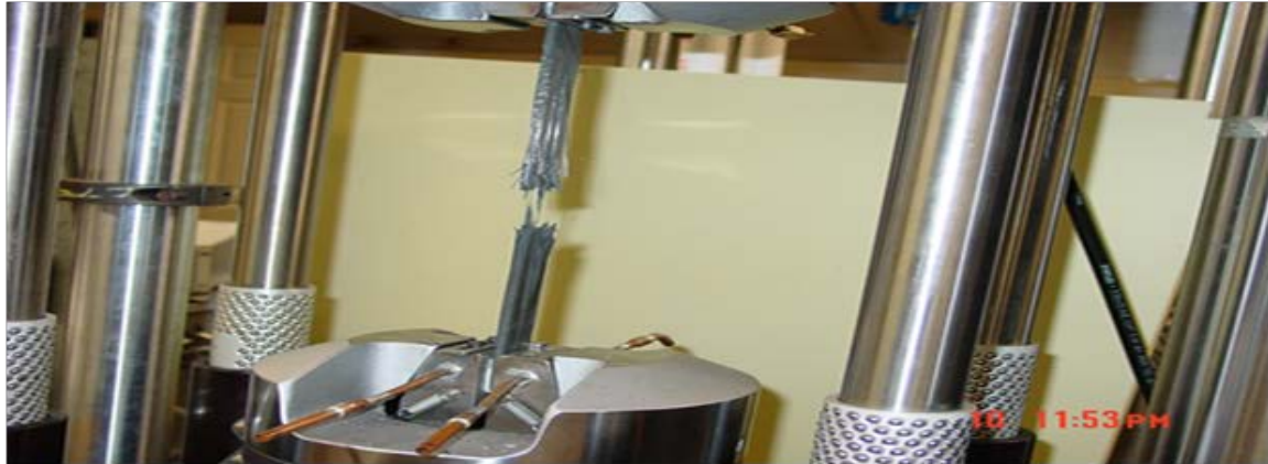
Figure 14 : Specimen Test Fixture after Fatigue Failure [41]
