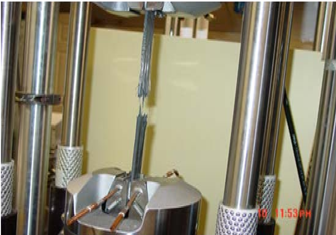
Figure 10 : Specimen Test Fixture after Fatigue Failure [41]
