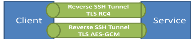
Figure 8. Increase Availability through Redundant Diversity
