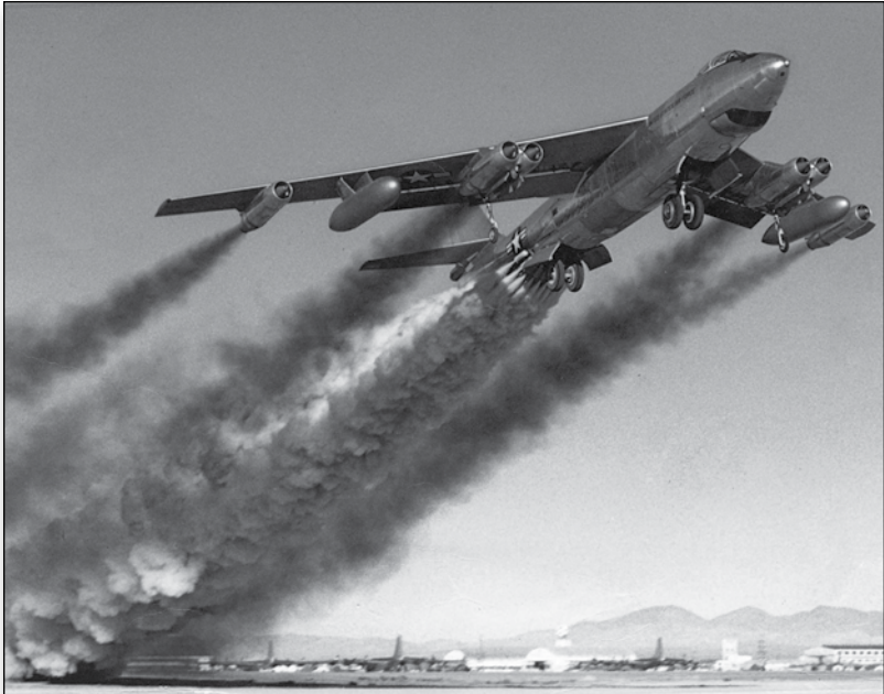
B-47s often used jet-assisted takeoff (JATO) bottles, which were jettisoned once in the air.
