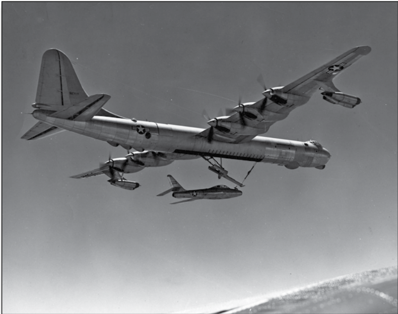
A YRB-36 carries a YF-84F in a trapeze during Project FICON to develop “parasite” fighters which would allow US bombers to penetrate Soviet air defenses.
