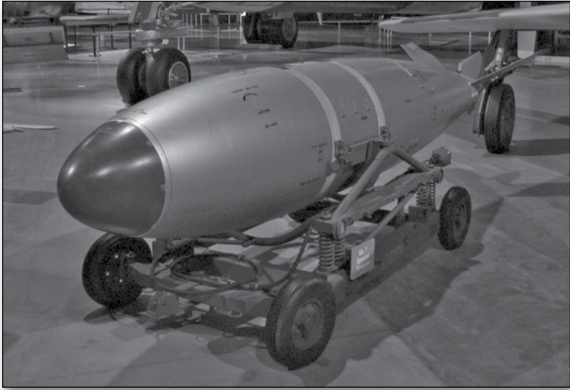
The Mark 7 "Thor" was the first tactical nuclear bomb adopted by US armed forces and was to be delivered using the toss method with the help of the low-altitude bombing system (LABS).
