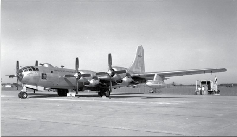
Boeing's B-50 Superfortress strategic bomber was a post-WWII revision of the B-29 Superfortress, fitted with more powerful Pratt & Whitney engines and among the last piston-driven bombers leading to the jet age.
