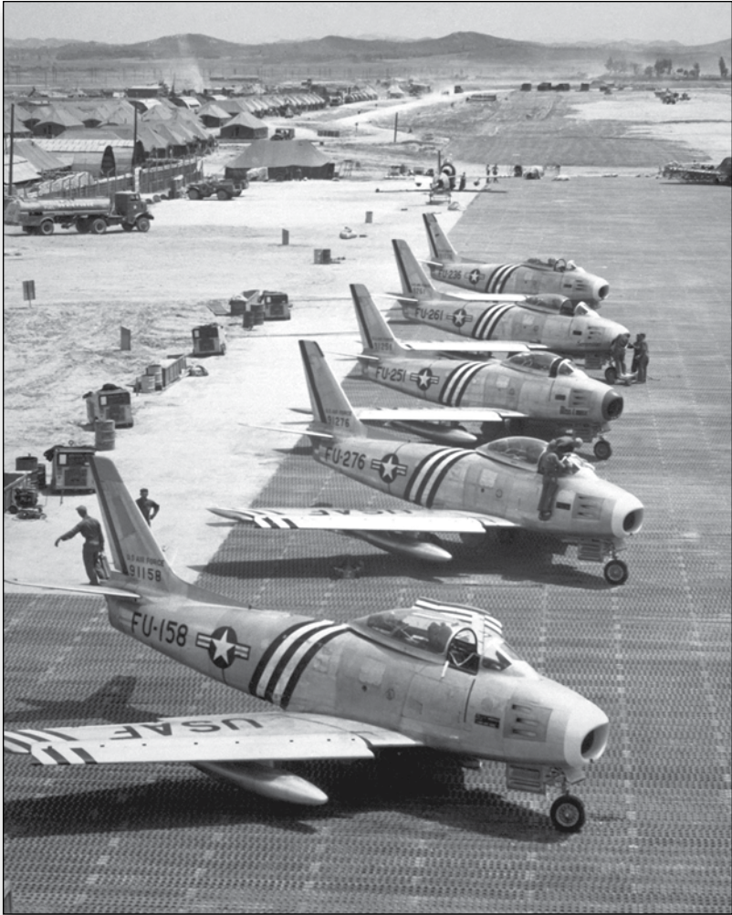
The North American F-86 Sabre was America's first swept-wing fighter, built to counter the similarly designed Soviet MiG-15 in high-speed dogfights during the Korean War.
