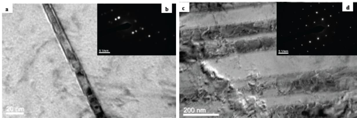
**Figure 9:** TEM images of 20% deformed 316 [111] single crystal samples
