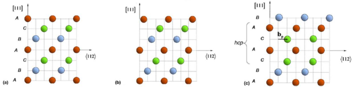
**Figure 3:** The schematic process of the martensitic transformation [8]
