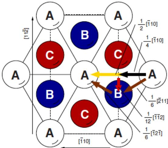
**Figure 5a:** Geometry of shear deformation on (111) planes[18].
