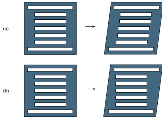
**Figure 5b:** The schematic view of possible deformation regimes: (a) affine shear, (b) the alias shear[18].
