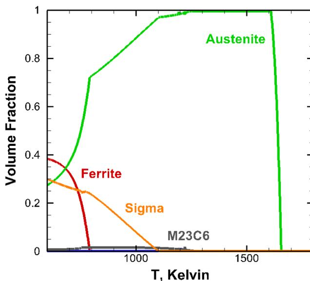
**Figure 10:** Phase analysis for Stainless Steel 316 with composition shown in **Table 1**.
