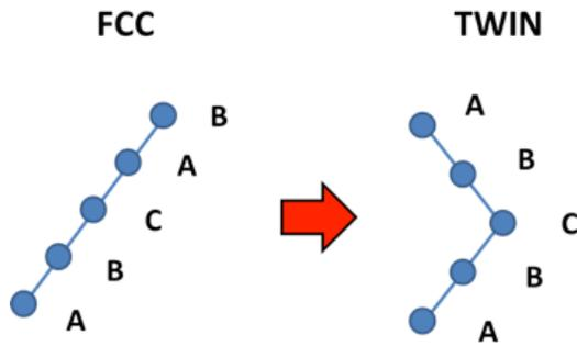
**Figure 1:** Schematic diagram of twinning in fcc systems.
