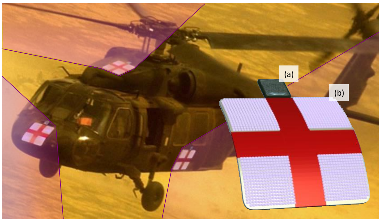
Figure 17. Concept of conformal Plasma-shell transceiver panel with large-area (a) detector and (b) emitter array, providing high-power 360° coverage for vehicles in a low-profile, light-weight package.
