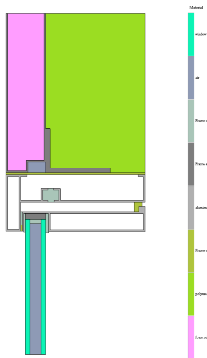
Figure 44. HEAT2 model of a window frame and joint in Bldg 2132, Fort Carson, CO.
