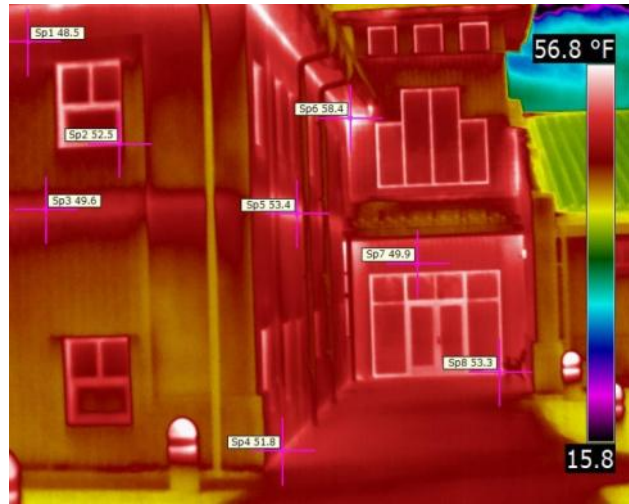
Figure 31. Window frame joints TB.
