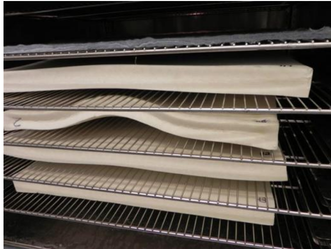
Figure 65. Post-conditioned polyurethane samples in the temperature and humidity chamber. Note: the middle samples are the post-conditioned samples.
