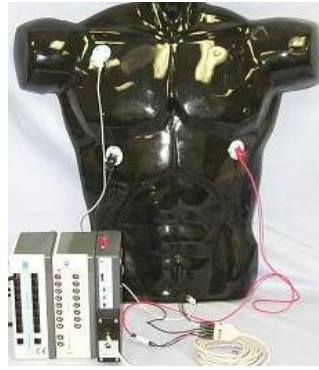
Figure 2: BIOPAC® hardware system showing placement of ECG electrodes.
