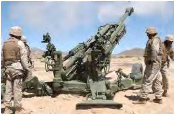
Figure 18 - M777 155mm howitzer 21 (Weight 9,300 lbs; Max Range 24Km-40Km; rof 2-5 rpm)
