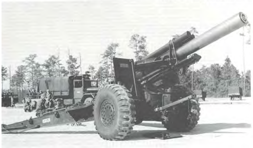
Figure 9 – M2 155mm gun (WWII) 11 (Weight 30,600 lbs; Maximum Range 23.2Km; rof 40 rph)
