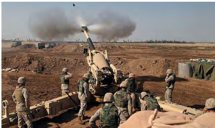
Figure 18 - M777 155mm howitzer 21 (Weight 9,300 lbs; Max Range 24Km-40Km; rof 2-5 rpm)
