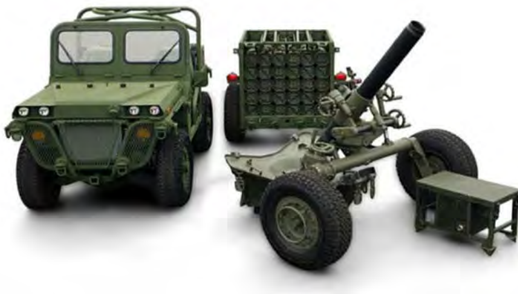
Figure 20 – M327 120mm mortar EFSS 23 (Weight 1,798 lbs; Maximum Range 8.2Km)
