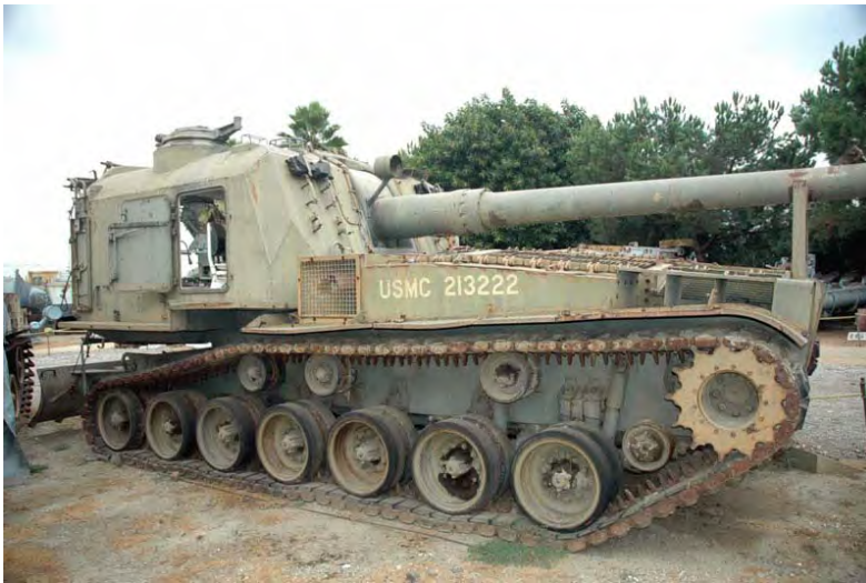
Figure 12- M110 8” howitzer 14 (Weight 62,390 lbs; Max Range 16.8Km-30Km; rof 2-4 rpm)
