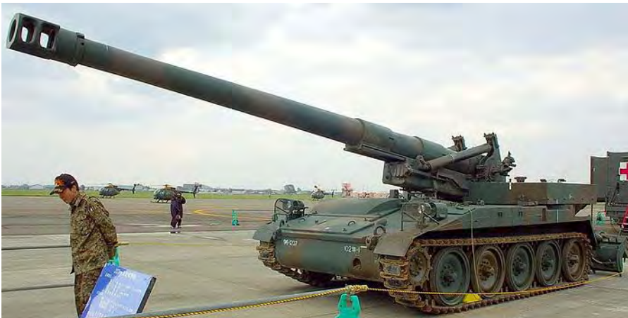
Figure 12- M110 8” howitzer 14 (Weight 62,390 lbs; Max Range 16.8Km-30Km; rof 2-4 rpm)
