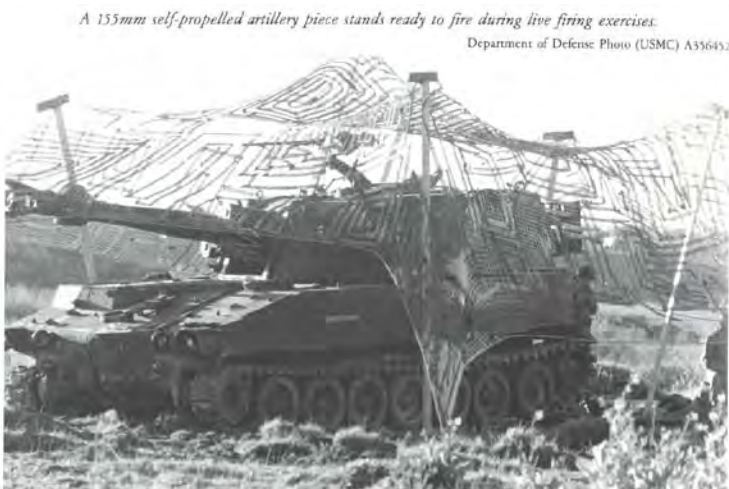
Figure 15 - M109 18 (Weight 27.5 tons; Maximum Range 18Km-30Km; rof 1-4 rpm)
