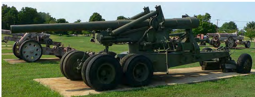
Figure 9 – M2 155mm gun (WWII) 11 (Weight 30,600 lbs; Maximum Range 23.2Km; rof 40 rph)
