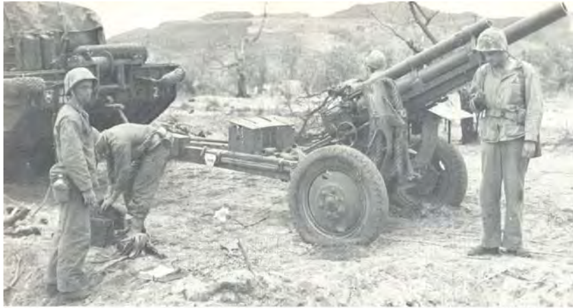
Figure 7 – M2 105mm howitzer 9 (Weight 5,000 lbs; Maximum Range 18.3Km)
