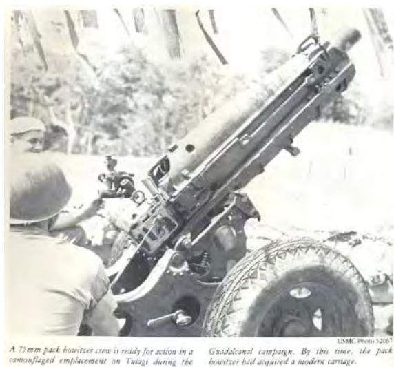
Figure 6 – M1 75mm pack howitzer 8 (Weight 1,000 lbs; Maximum Range 8.8Km; rof 3-6 rpm)
