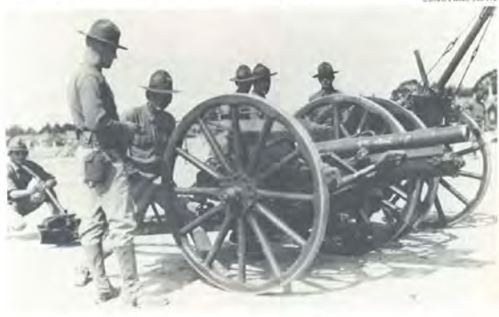
Figure 3 - 7 inch gun 4 (Weight 32 tons; Maximum Range 15Km-24Km) 5
