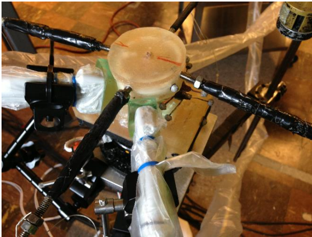
Figure 9. The lower vertebral body of the FSU was mounted in PMMA and attached to a plate fixed on a tripod. Four hydraulic pistons were rigidly attached to the PMMA to allow the application of force couples that induced pure flexion-extension or lateral bending moments to the FSU. The dual ultrasound probes were oriented to image the facet joints and spinous processes of C6-7.
