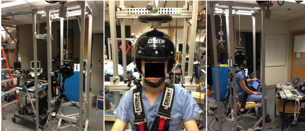
Figure 23 (a) Solenoid powered traction system for applying cyclic loads in-vivo: a programmable DC power supply is used to power a solenoid that applies a variable traction force via two fixed pulleys to a fixed weight attached to the top of the helmet; (b) front view (c) and side view demonstrating restraints and dual ultrasound probes positioned on the subjects neck anteriorly and posteriorly in a fixed orientation.
