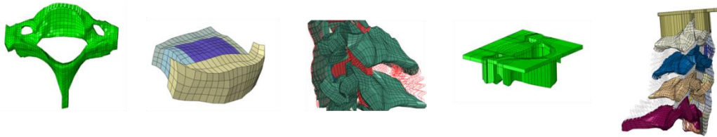
Figure 25 Finite element representations of subaxial cervical vertebra (left, as viewed from top), intervertebral disc (second from left, axial view), facet joints (third from left, sagittal view), loading device (fourth from left) and the sagittal view of the C4-C7 spinal column with the loading device at the superior end (right).
