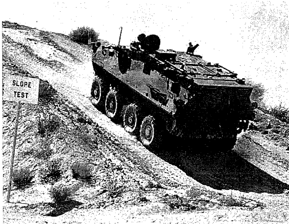
"Yermo Annex. A rebuilt Light Armored Vehicle Mortar (LAV-M) is run through an inclined road test by maintenance crews from the Defense Logistics Agency." Photographer's Name: GS-09 Curtis Lambert Location: USMC LOGISTICS BASE, BARSTOW Date Shot: 8/25/1993 Date Posted: unknown VIRIN: 930825-M-2375L-
