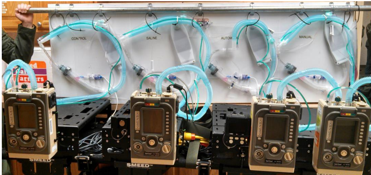
Figure 1. Model system including model trachea, ETT, test lungs, and ventilators.
