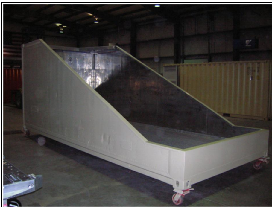
Figure 10. Completed field lysimeter prior to transport to the CAFB M-60 range.
