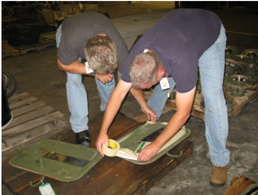
Masking spall liner prior to abrasive blasting of high hard hatches
