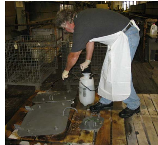
Application of chemical pretreatments
